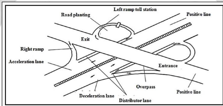
Figure 5: Geometric elements of an interchange ramp. [18].
