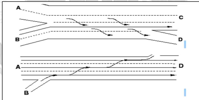
Figure 4: Type C Weaving Configuration.[17].
