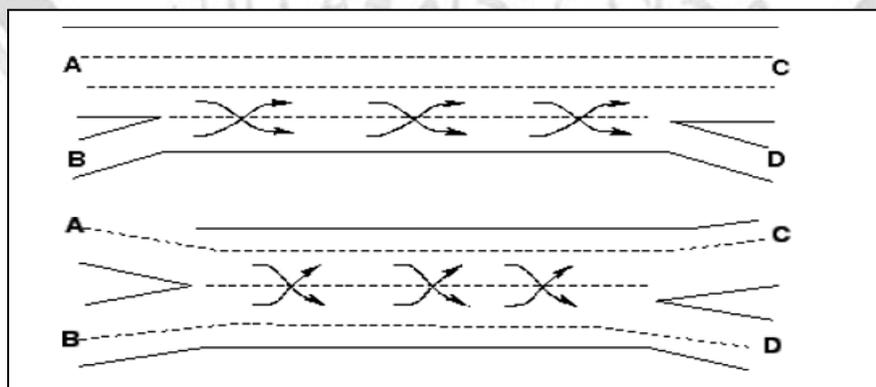
Figure 2: Type A Weaving Configuration. [17].
