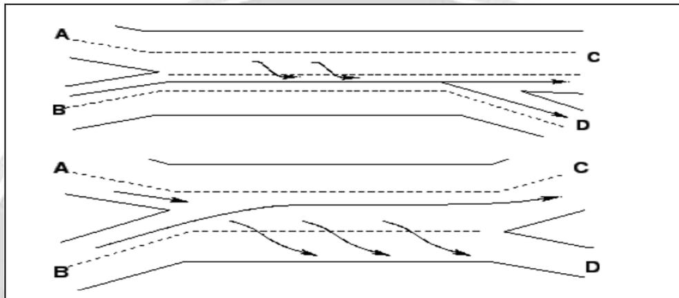
Figure 3: Type B Weaving Configuration. [17].
