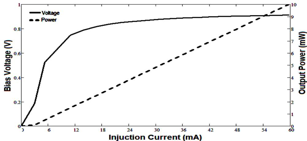
**Figure (6) Voltage, current and output power characteristics.**
