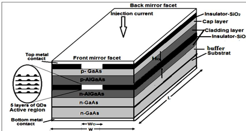
Figure (3) Schematic illustration of the QD-LD structure.
