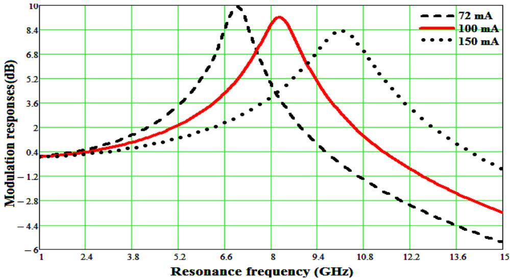
Figure (10) Modulation responses at several injected currents.
