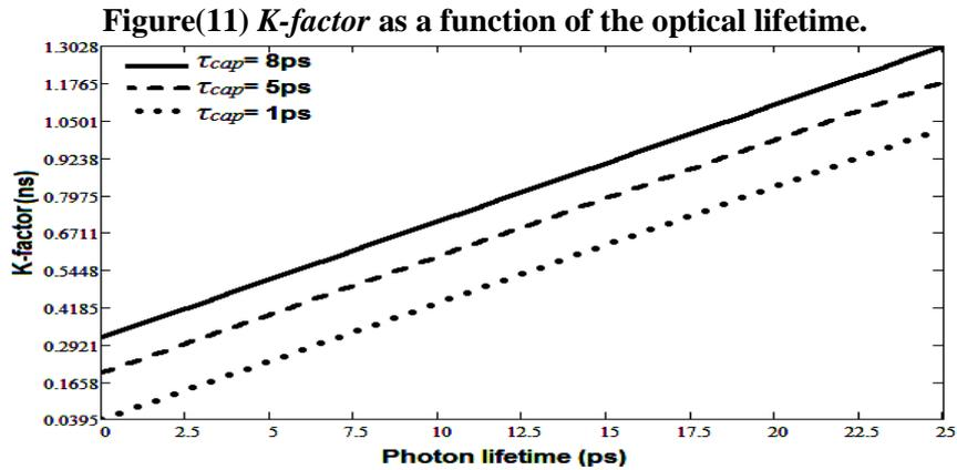
**Figure (12) K-factor as a function of the lifetime at different value of the capture times.**
