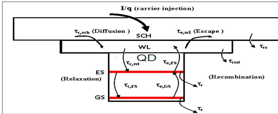
**Figure (1) Schematic diagram of the components in the InAs-QD, InGaAs-WL and GaAs-SCH material system of QD-LD for the conduction band energy levels [6].**
