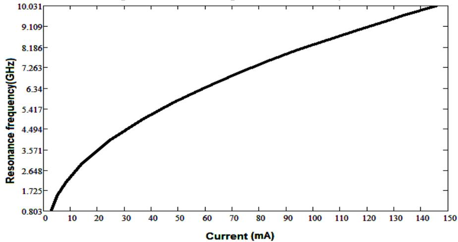
**Figure (8) Resonance frequency of the modulation response versus the injection current.**
