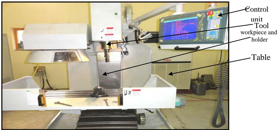
Figure (1) shows CNC Milling machine (model KM-80D).
