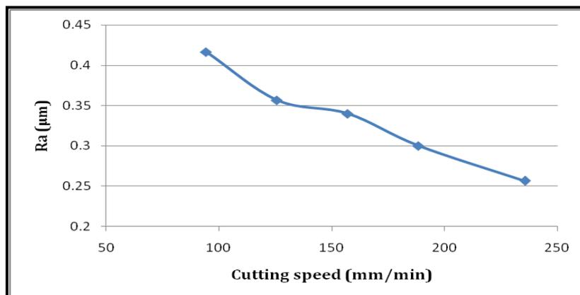
**Figure (5) Effect of cutting speed on surface roughness.**
