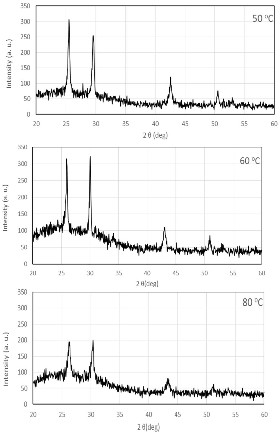
**Figure (1) X-ray diffraction spectrum of PbS thin films for various substrate temperature.**
