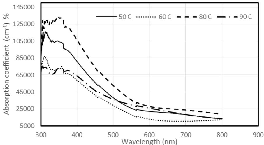
**Figure (3) Absorption coefficient as function of wavelength for PbS films with different substrate temperature.**
