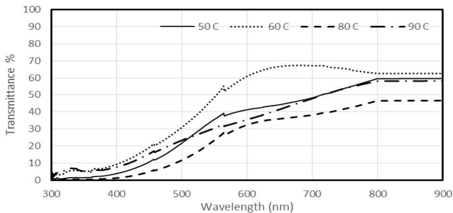
**Figure (2) Transmission as function of wavelength for PbS films with different substrate temperature.**
