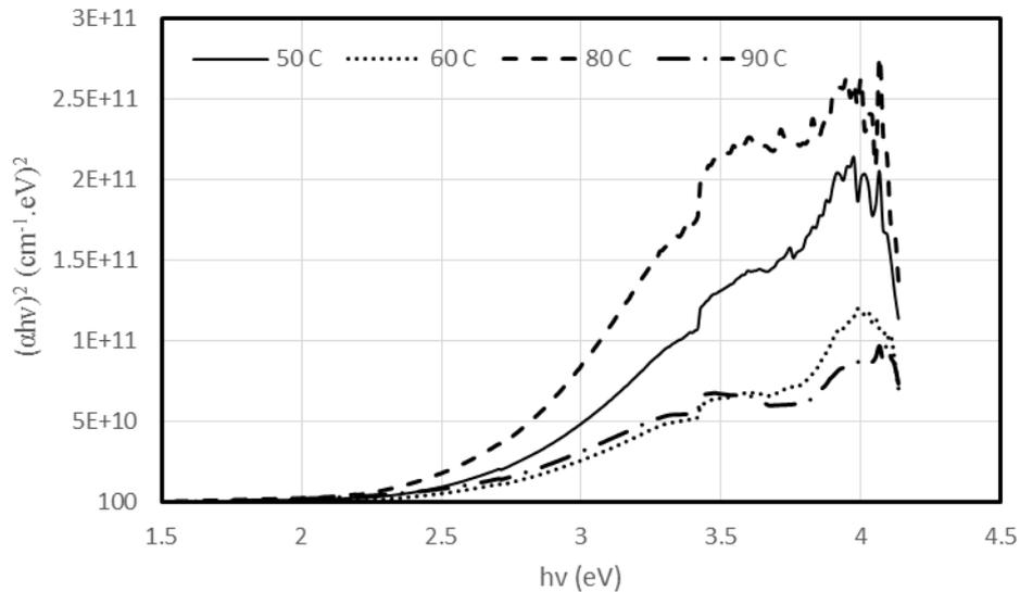
Figure (4)  $(\alpha hv)^2$  verity as function of energy for PbS films with different substrate temperature.
