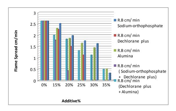
Figure (4) Variation of flame spread with weight percentages of additives for EP
