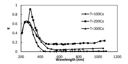
Figure (4): Extinction coefficient of CdO films annealed at different temperatures as a function of wavelength.
