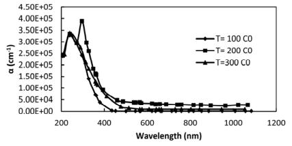
Figure (3): absorption coefficent of CdO films annealed at different temperatures as a function of wavelength
