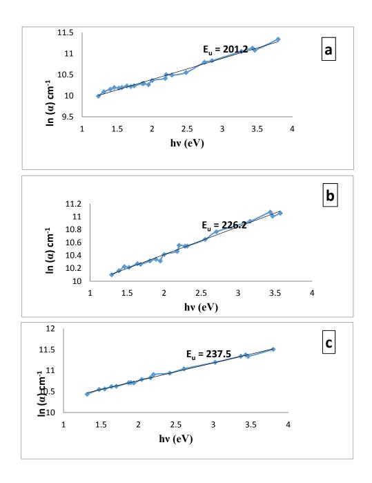
Figure(6): Variation of (ln  $\alpha$ ) Vs (hv) of CdO films annealed at different temperatures a)100 C°, b)200 C°, and c)300C°.
