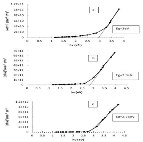
Figure(5): Variation of  $(\alpha hv^2)$  Vs (hv) of CdO films annealed at different temperatures a)100 C°, b)200 C°, and c)300C°.
