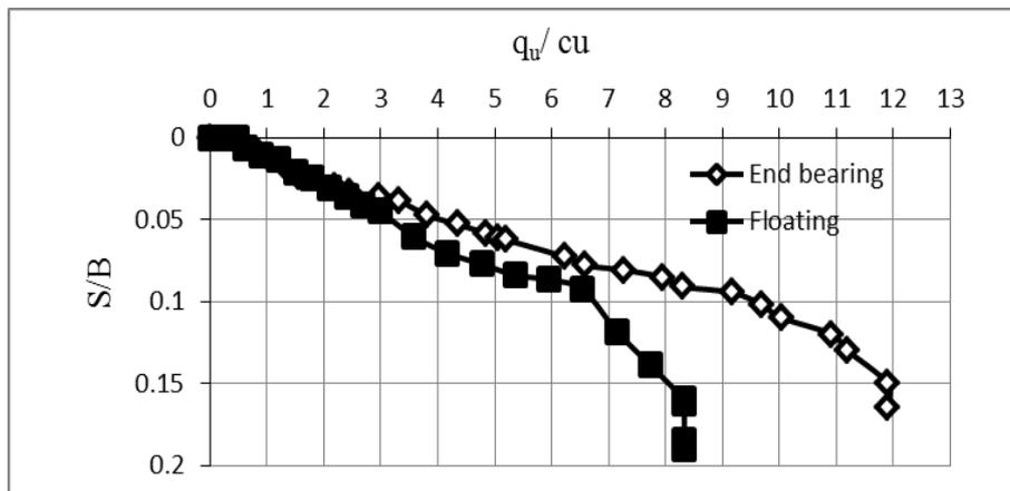
Figure (9) Pressure –settlement curve for a footing resting on soft clay treated by four stone columns group.
