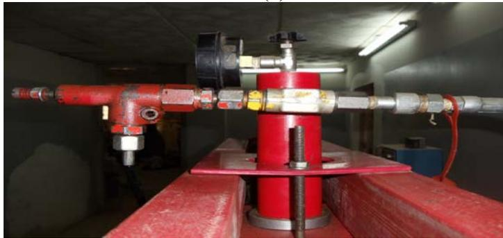
(c) Side view of the axial loading system.
