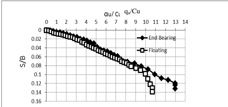
Figure (11) Pressure –settlement curve for a footing resting on soft clay treated by six stone column group.
