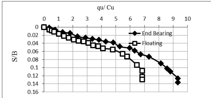
Figure (8) Pressure –settlement curve for a footing resting on soft clay treated by three stone column group.
