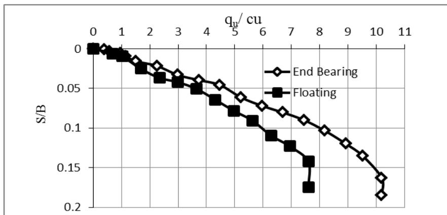
Figure (7) Pressure –settlement curve for a footing resting on soft clay treated by two stone column group.
