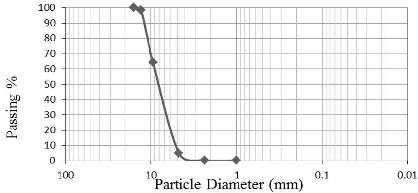
Figure (2) Grain size distribution of the crushed stone material.
