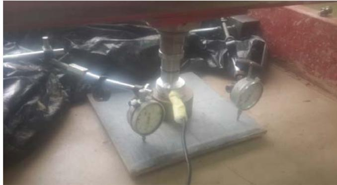
**Plate (5) Loading of four-stone column group.**
