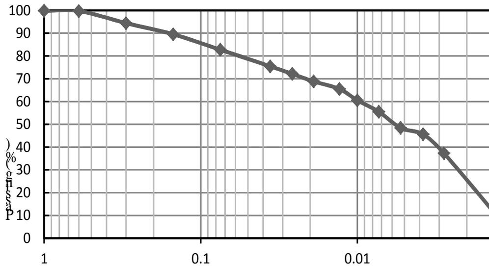
**Figure (1) Particle size distribution of the soft soil used.**
