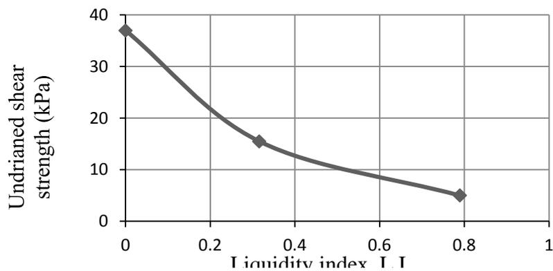
Figure (4) Variation of the undrained shear strength with liquidity index for the remolded clay after (5) days.
