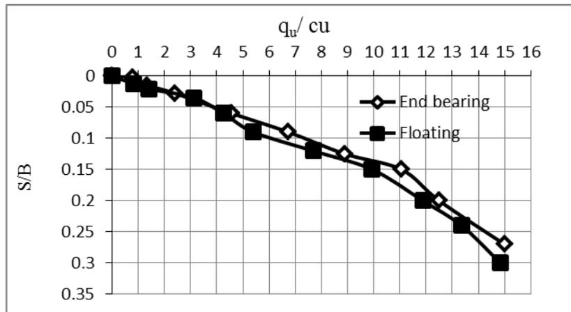
Figure (6) Pressure –settlement curve for a footing resting on soft clay treated by single stone column.
