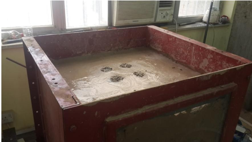
Plate (1) Four-end bearing stone column group model.
