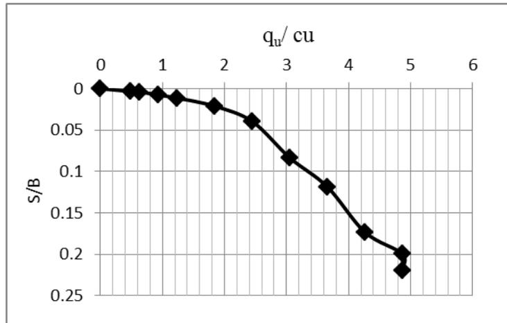
Figure (5) Pressure –settlement curve for a footing resting on untreated soil.
