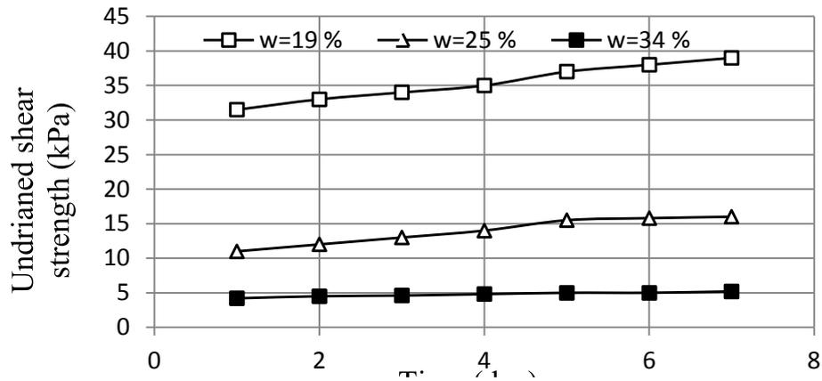
Figure (3) Variation of the undrained shear strength with time for different water contents of the remolded clay.
