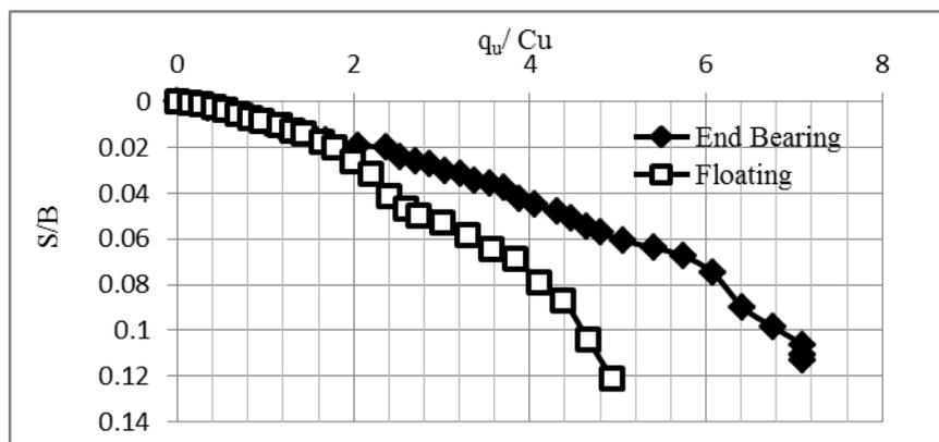
Figure (10) Pressure –settlement curve for a footing resting on soft clay treated by five stone column group.
