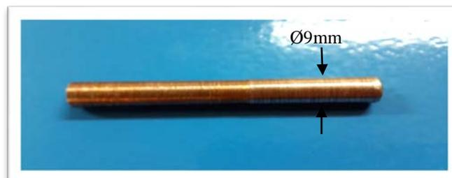
**Figure(6). Copper electrode before machining.**
