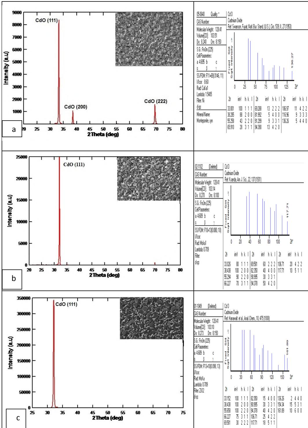
Figure (1a, b and c) shows XRD of (CdO) films deposited normally and obliquely ( $\theta=0^\circ$ ,  $\theta=50^\circ$  and  $70^\circ$ ) respectively.
