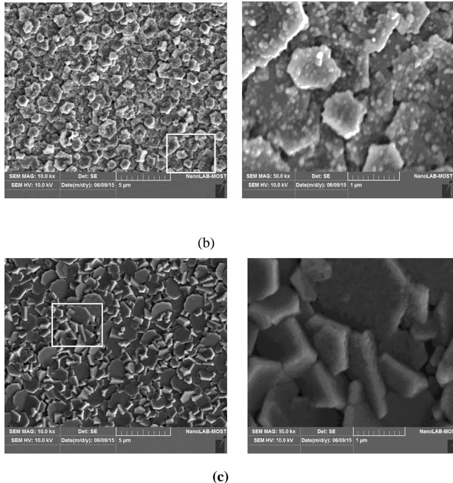
Figure (2) SEM images of cadmium oxide nanofilm evaporated at (a) normal 0° (b) 50° and (c) 70° angles of incidence.
