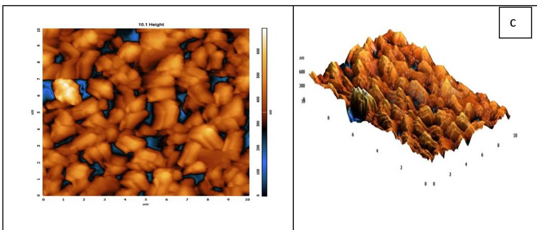
**Figure (3) AFM images of evaporated thin films deposited at (a) 0°, (b) 50° and (c) 70° angles of incidence.**
