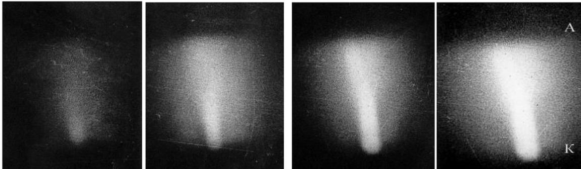
**Fig (4): Frame photographs illustrating the formation and growth of the spark channel**
