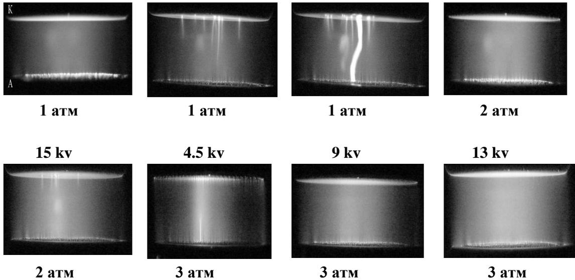
**Fig (2): Time –integral photographs of the glow under different initial condition plane stainless –steel electrodes (the solid cathode, and the grid anode). The gap length  $d=1$  cm.**
