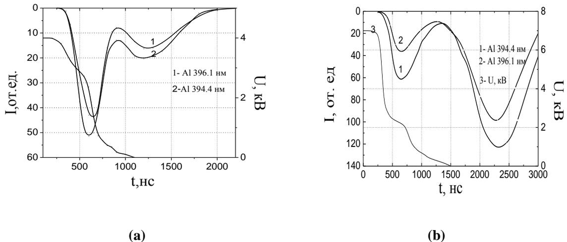
**Fig (3): Typical time dependences of the intensities of aluminum spectral lines emitted from the cathode at discharge voltage of (a) 4 and (b) 7 kV Hemispherical aluminum electrodes with a curvature radius of  $R=30$  cm, the gap length is  $d=1$  cm ,and the gas pressure is  $p=1$  atm.**
