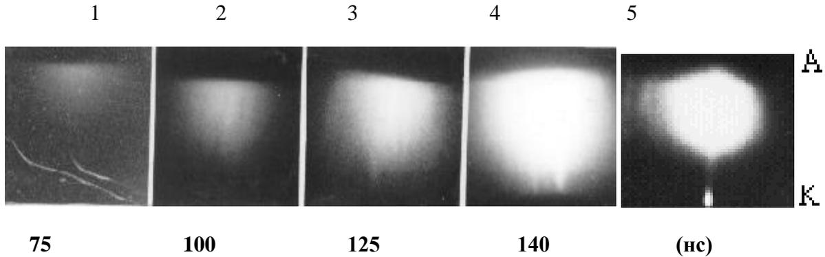
**Fig (1):** Frame photographs illustrating the formation of a VD with external preionization (the preionization source is aside) in He discharge voltages of  $U_0 = 15$  kV (frames 1 – 4),  $U_0 = 18$  kV (frames – 5) (aluminum electrodes with a curvature radius of 30 cm, the gap length is  $d=1$  cm and  $p=1$  atm).
