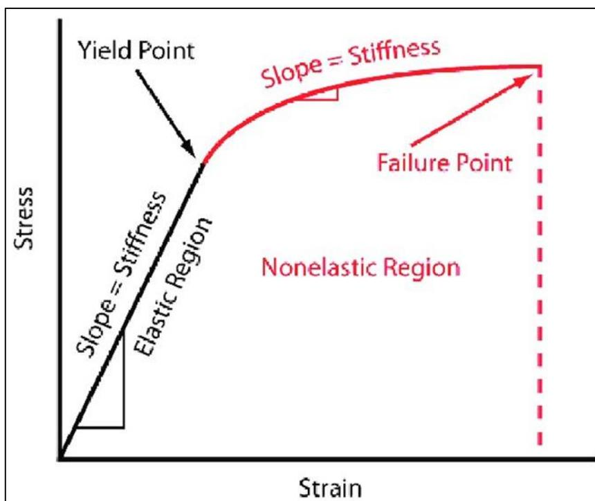
**Fig. 6.** Ductile Material Stress-Strain Curve
