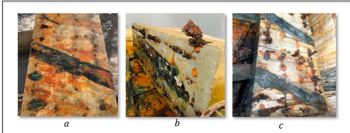
**Fig. 5** (a. weak corrosion, b. moderate corrosion, and d. sever corrosion)
