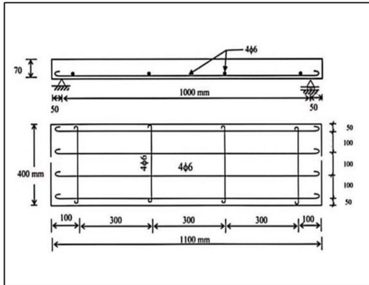
**Fig. 1.** Slab Details (dimensions, steel diameter, and spacing)
