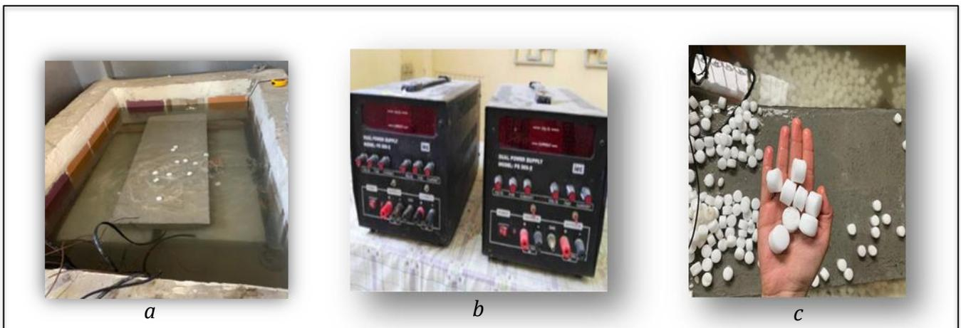
**Fig. 2** (a. corrosion basin, b. power supply, and c. NaCl used)
