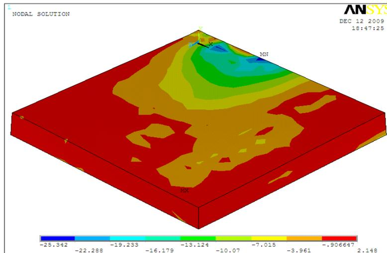
**Figure (6) Variations in stress in X-direction for control slab (SL)**
