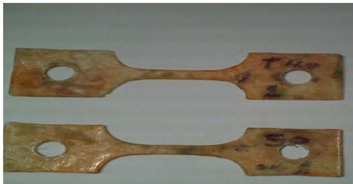
Figure.(5) Photograph of composite creep test specimen
