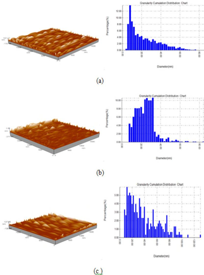
**Figure (4) AFM images of Silver films deposited on glass substrate at vacuum chamber pressure  $10^{-5}$  mbar, and substrate temperature(  $300^{\circ}\text{C}$  )at different Laser fluence: (a)  $0.4 \text{ J/cm}^2$  (b)  $0.6 \text{ J/cm}^2$  (c)  $0.7\text{J/cm}^2$ .**
