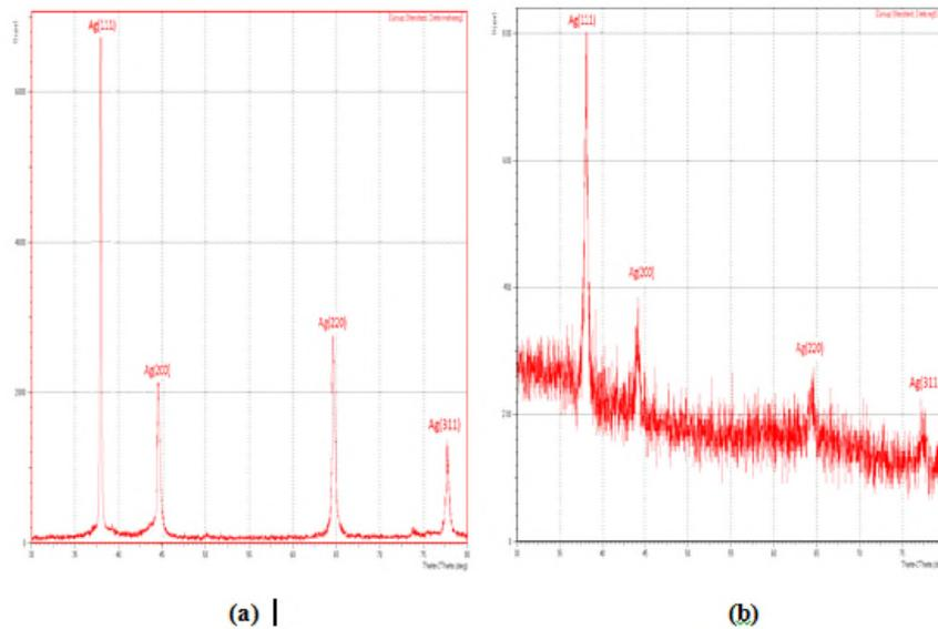
**Figure (2) X-Ray diffraction for Ag (a) Ag target before ablation (b) Ag thin film.**
