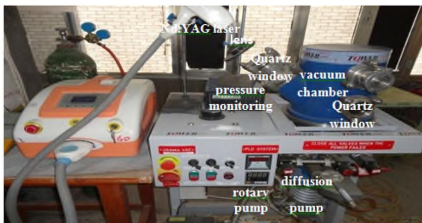
**Figure (1) PLD system Set-Up**
