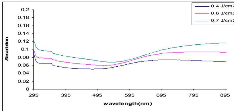
**Figure (7) Absorbance spectrum of nanostructure Au thin films at different laser fluence (0.4, 0.6 and 0.7) J/cm<sup>2</sup>.**
