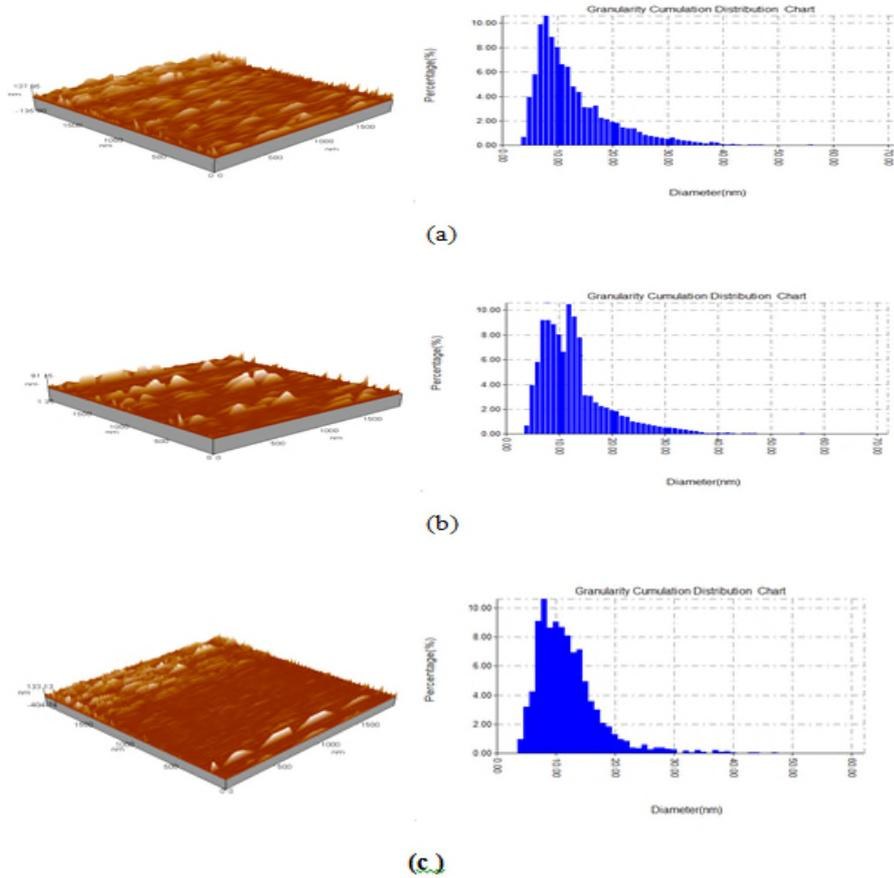
**Figure (5)** AFM images of gold films deposited on glass substrate at vacuum chamber pressure  $10^{-5}$  mbar, and substrate temperature(  $300^{\circ}\text{C}$ )at different Laser fluence: (a)  $0.4 \text{ J/cm}^2$  (b)  $0.6 \text{ J/cm}^2$  (c)  $0.7 \text{ J/cm}^2$ .
