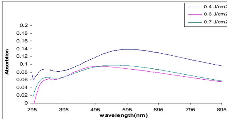
**Figure (6) Absorbance spectrum of nanostructure Ag thin films at different laser fluence (0.4, 0.6 and 0.7) J/cm<sup>2</sup>.**
