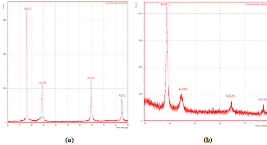
**Figure (3) X-Ray diffraction for Au (a) Au target before ablation (b) Au thin film.**
