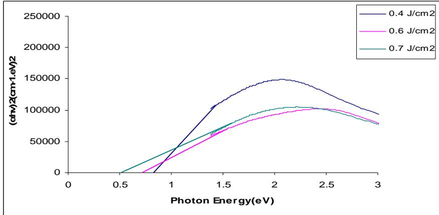
**Figure (8) Energy gap of Ag thin films at different laser fluence (0.4, 0.6 and 0.7)  $J/cm^2$ .**
