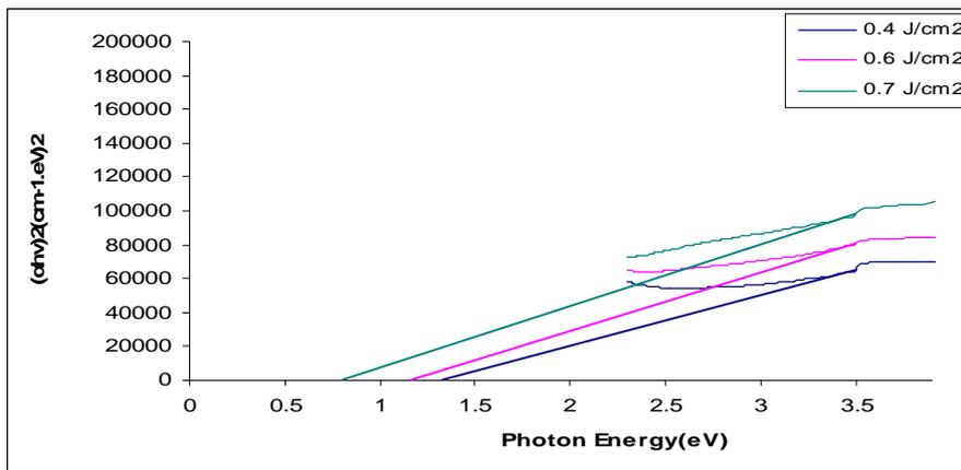
**Figure (9) Energy gap of Au thin films at different pulses energy (60, 80 and 100)mJ.**
