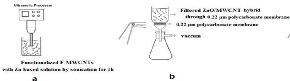
Figure(1): Schematic diagram of method for preparing ZnO/MWCNTs hybrid .
