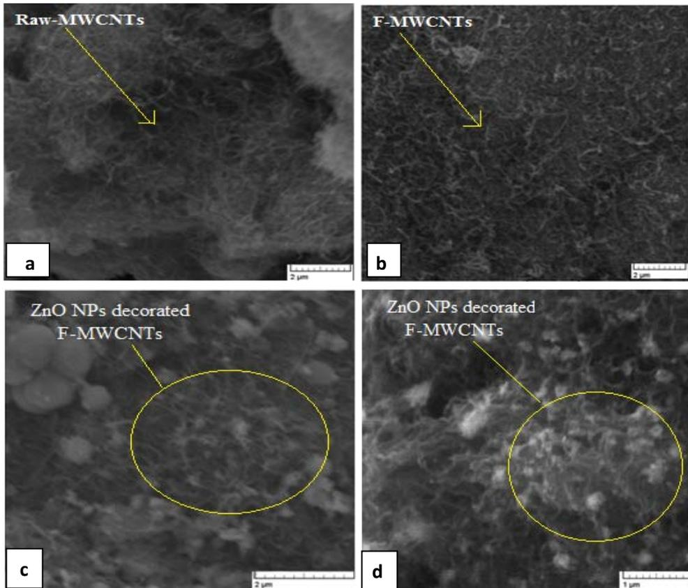
Figure(2): SEM images of a) raw-MWCNTs, b) F-MWCNTs and c,d,) ZnO/MWCNTs hybrid at different magnifications.
