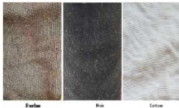
Figure 1: Reinforcing materials utilized in this Study.
