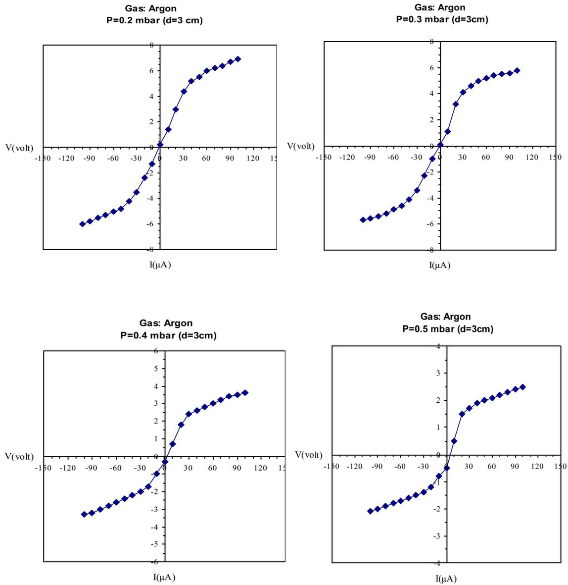
Fig.(6) I – V characteristics of double probe in different pressure ranges.
