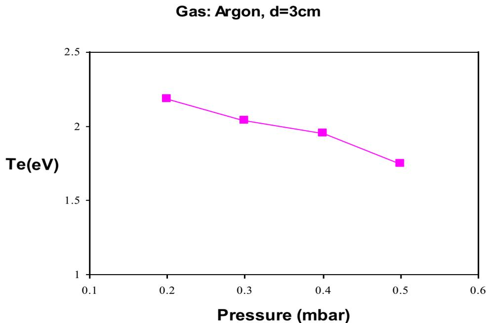
**Figure (7): The relation between temperature of electron as a function to the pressure.**
