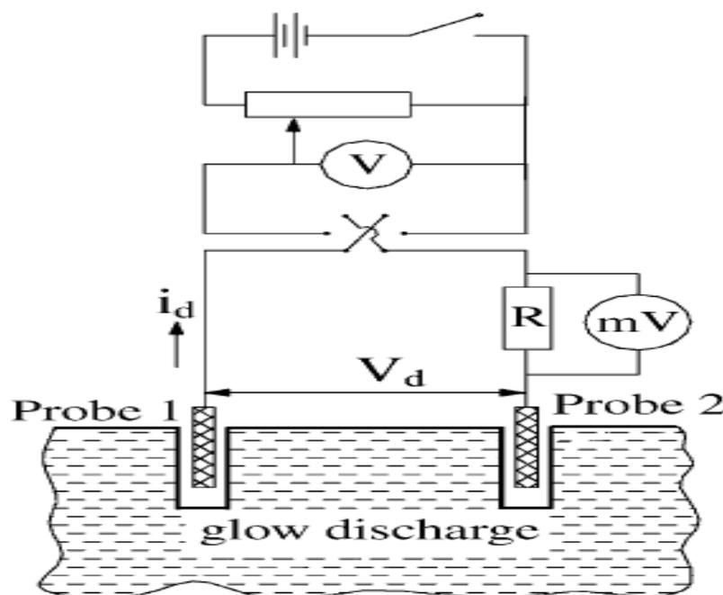
Fig.(2): Basic double probe circuit [12].
