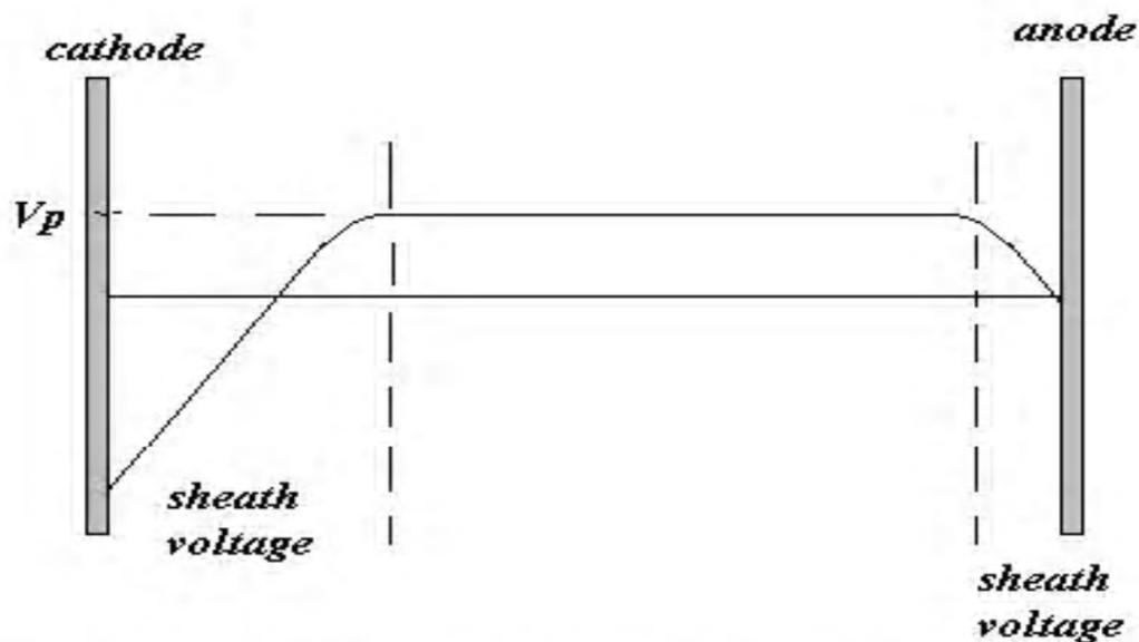
Fig.(1): Voltage distribution in a DC glow discharge process.
