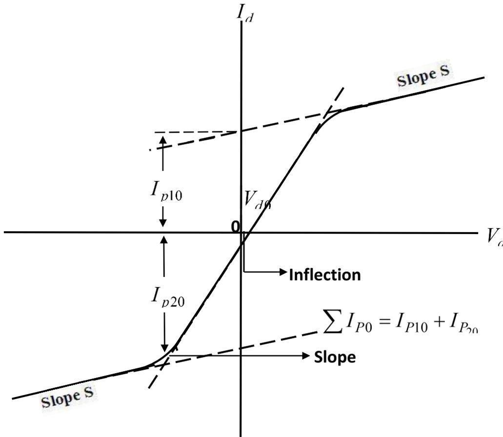
Fig.(3): Schematic diagram of the double probe characteristic [10].
