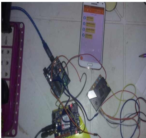
Figure 12. The implemented SIM900 Board
