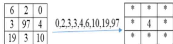
Figure (4): Example of 3*3 of Median Filter.
