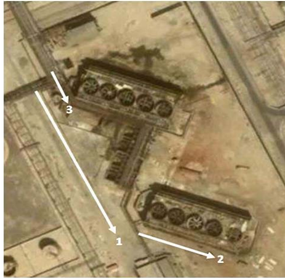
Figure (4): Unit no.1 with GPR profiles
