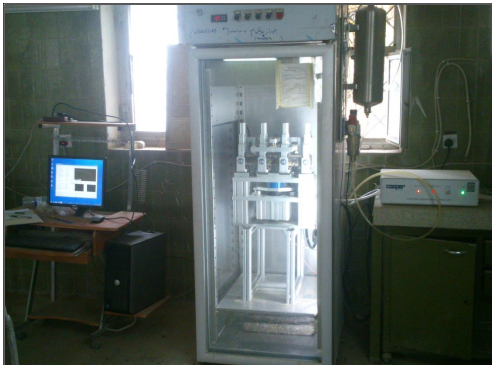
Figure 4. Flexural fatigue testing equipment (NCCLR laboratory, Baghdad).
