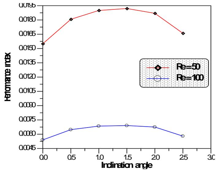
Fig. 7 Variation of performance index with inclination angle for square channels
