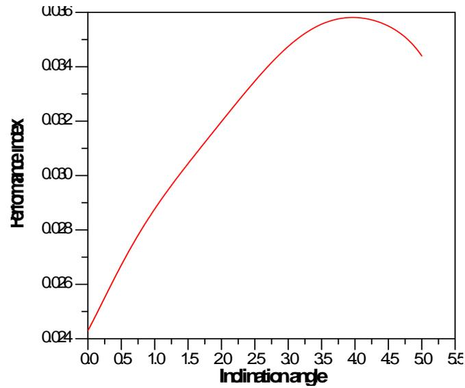
Fig. 15 Variation of performance index with angle for rectangular channels (AR=1.5 & Re=50 )
