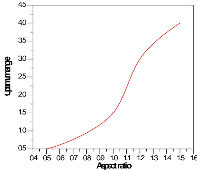
Fig. 17 Variation of optimum angle with aspect ratio for rectangular channels
