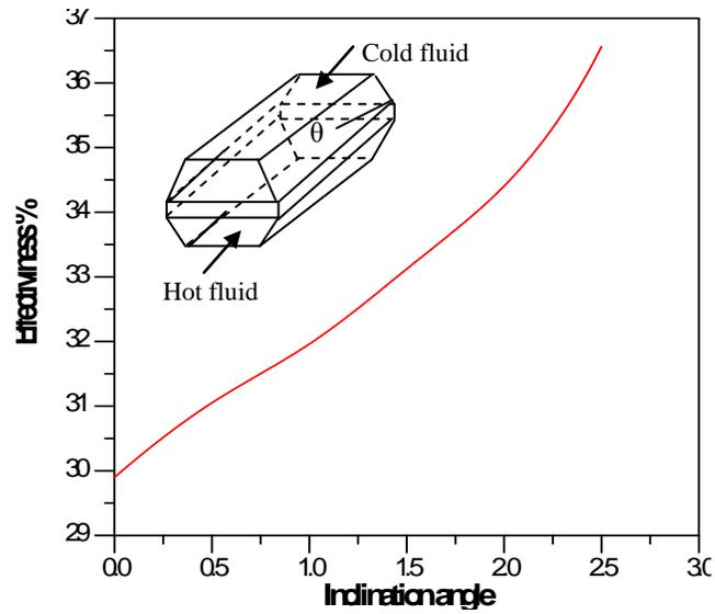
Fig. 19 Variation of effectiveness with inclination angle for trapezoidal channels (Re = 50)
