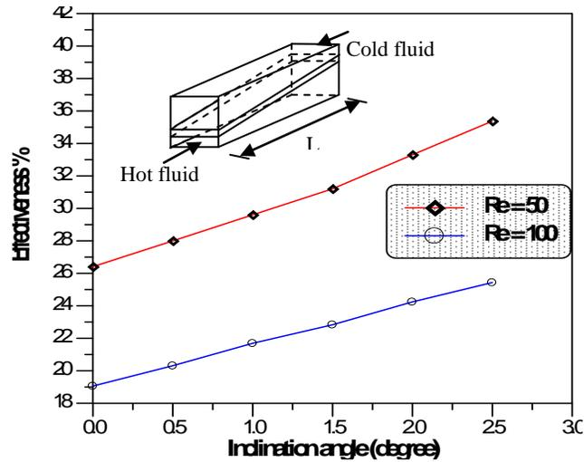
Fig. 5 Variation of effectiveness with inclination angle for square channels
