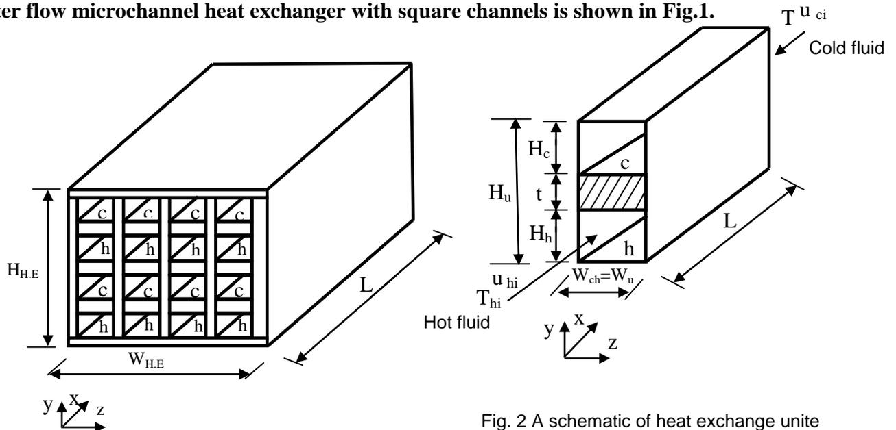
Fig. 1 A schematic model of the counter flow MCHE
