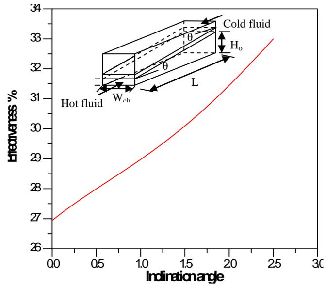
Fig. 9 Variation of effectiveness with angle for rectangular channels (AR=0.5 and Re =50)
