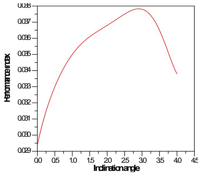
Fig. 13 Variation of performance index with angle for rectangular channels (AR=1.2 & Re = 50 )
