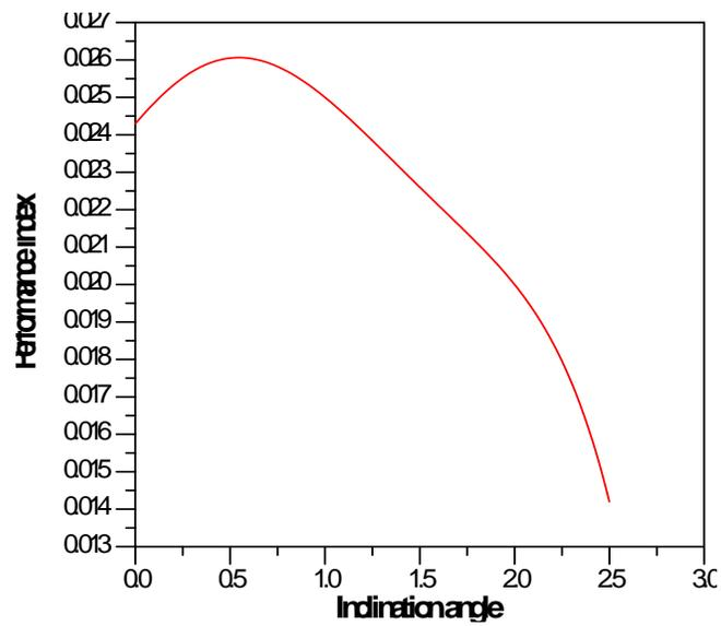
Fig. 20 Variation of performance index with inclination angle for trapezoidal channels (Re = 50)
