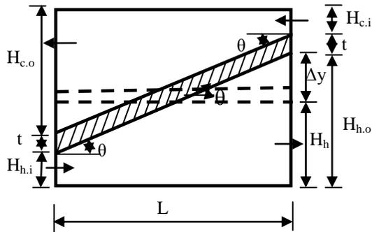
Fig. 3 Two-dimensional schematic of the heat exchange unit with variable area channels.
