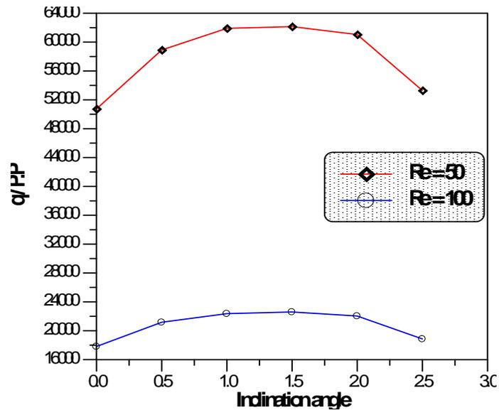
Fig. 8 Variation of heat transfer rate over pumping power ratio with inclination angle for square channels
