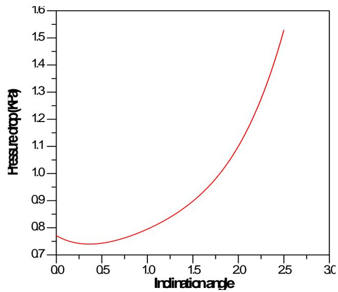
Fig. 10 Variation of pressure drop with angle for rectangular channels (AR=0.5 and Re = 50)
