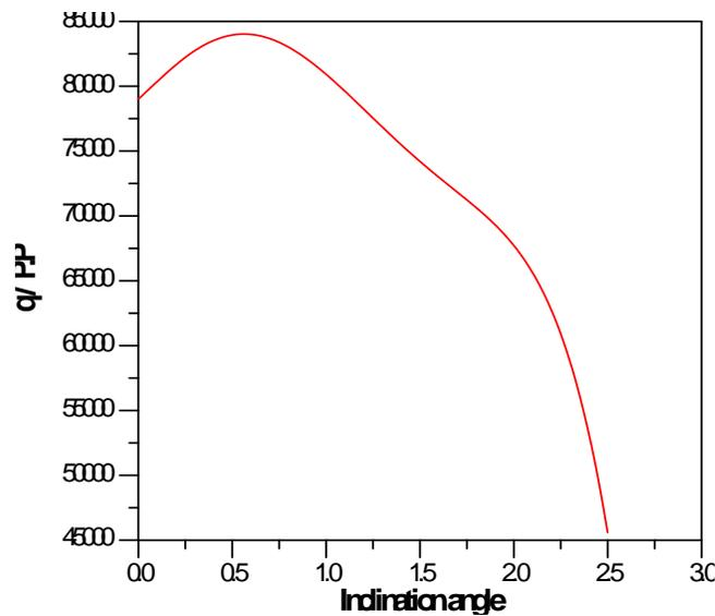
Fig. 21 Variation of heat transfer rate over pumping power with inclination angle for trapezoidal channels ( $Re = 50$ )
