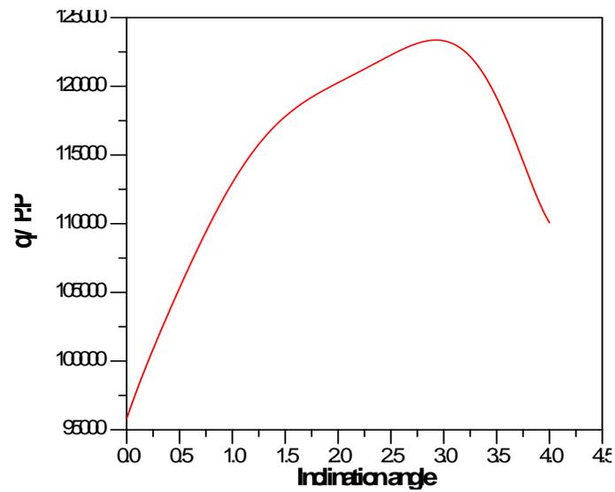
Fig. 14 Variation of heat transfer rate over pumping power with Angle for rectangular channels (AR=1.2 & Re = 50 )
