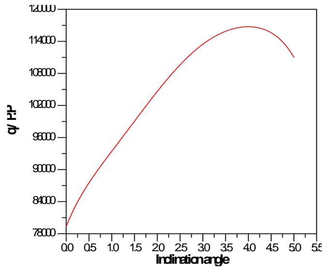
Fig. 16 Variation of heat transfer rate over pumping power with angle for rectangular channels (AR=1.5 & Re = 50 )
