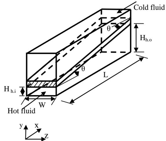
Fig. 4 3D schematic of the heat exchange unit with variable cross-sectional area channels
