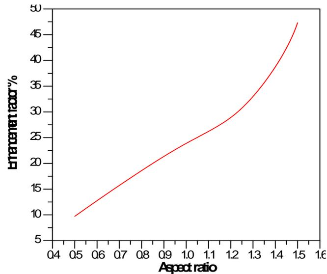
Fig. 18 Variation of enhancement in performance index with aspect ratio for rectangular channels
