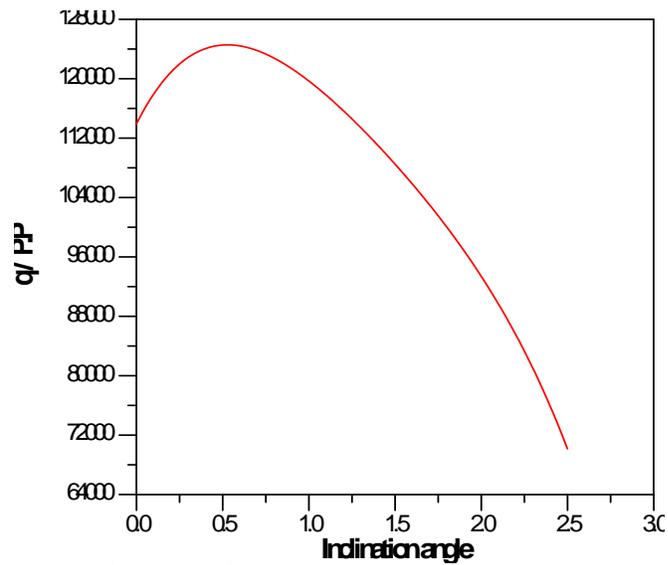
Fig. 12 Variation of heat transfer rate over pumping power with inclination angle for rectangular channels (AR=0.5 & Re = 50)
