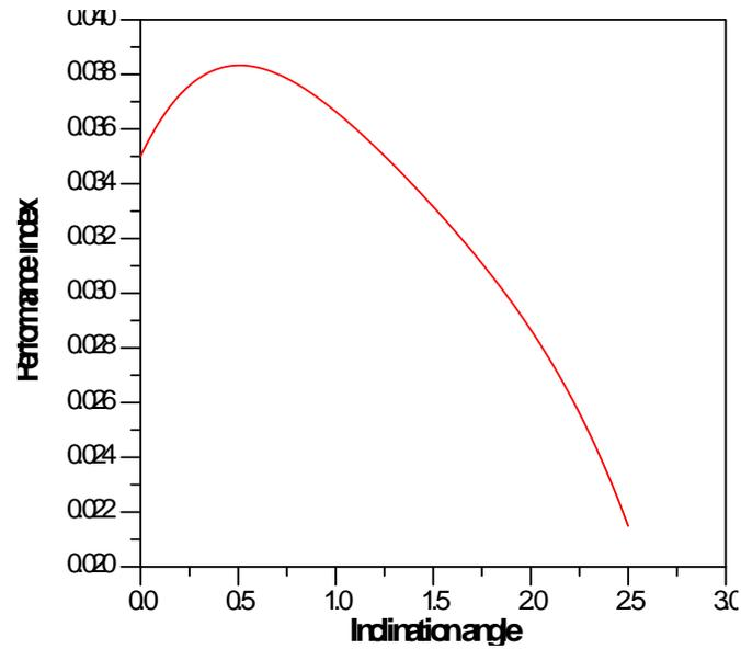
Fig. 11 Variation of performance index with angle for rectangular channels (AR=0.5 & Re =50)
