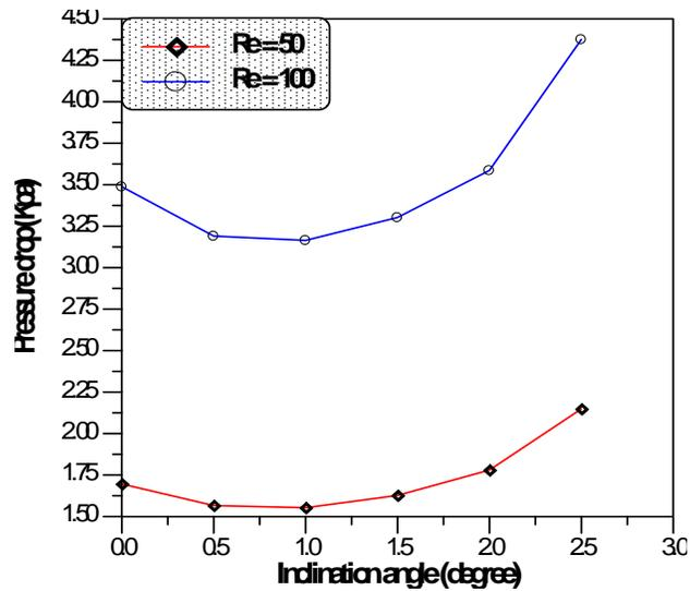
Fig. 6 Variation of pressure drop with inclination angle for square channels
