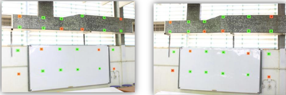
Fig.3 : Stereo pair of digital photos picking up by mobile phone Camera
