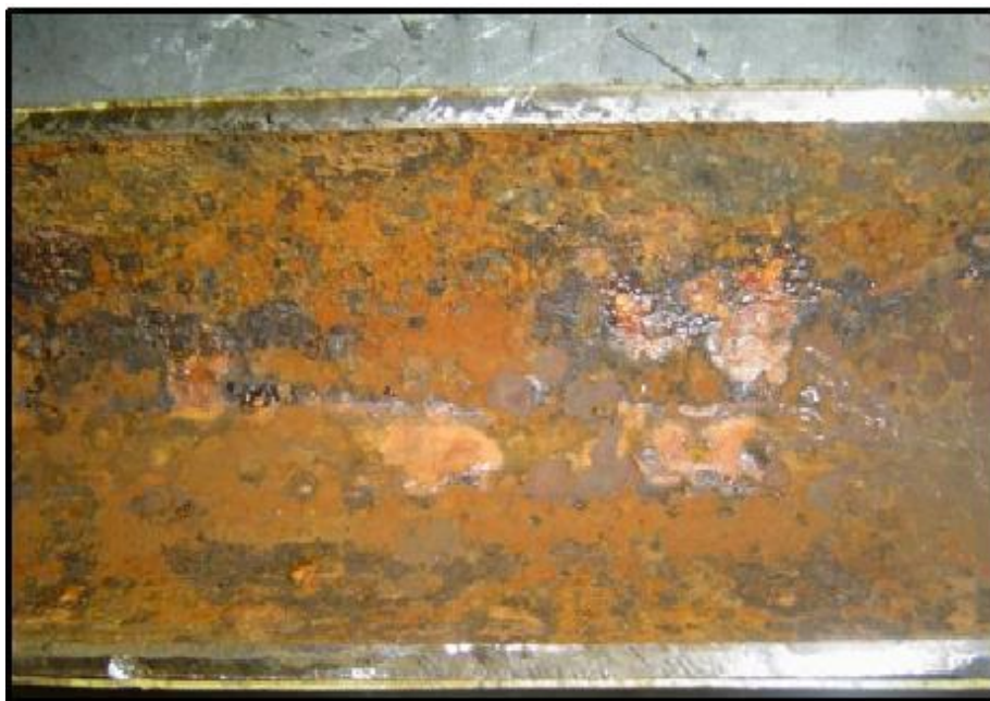
Figure 1. Internal corrosion of water injection pipeline.
