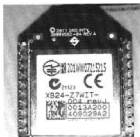
Figure 3. XBee address printed on the back of the module
