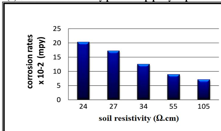
Figure (4) Average corrosion rate as a function of soil resistivity at different exposure times (24, 48, 72) h and surface area of 3 cm<sup>2</sup>.
