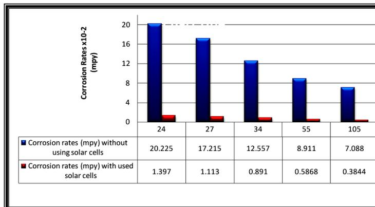
Figure (6) Effect the cathodic protection on average corrosion rates with using solar cells source for buried steel pipelines at different soil resistivity and surface area of (3cm<sup>2</sup>).
