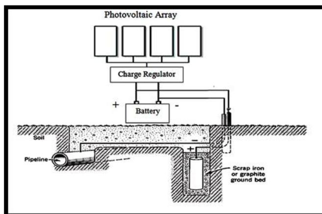
**Figure (1) Supplied solar energy for cathodic protection installation [4].**
