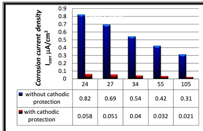
Figure (5) Effect the cathodic protection on corrosion current density of buried steel pipeline at different soil resistivity.
