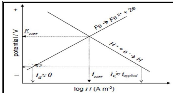
Figure (2) Polarization curve to determine values of ( $I_{corr}$ ,  $E_{corr}$ ) [1].
