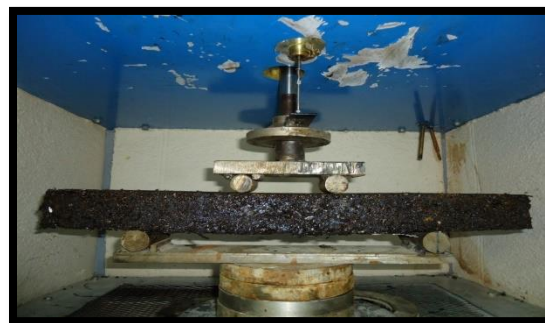
Figure 6. Flexural bending fatigue test.
