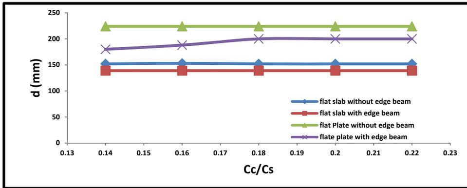
Figure (7): Effective Depth Versus Material Costs Ratio
