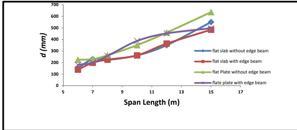
Figure(9): Slab Effective Depth Versus Span Length
