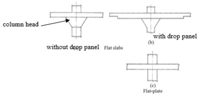
Figure (1) Flat Slab and Flat Plate Systems
