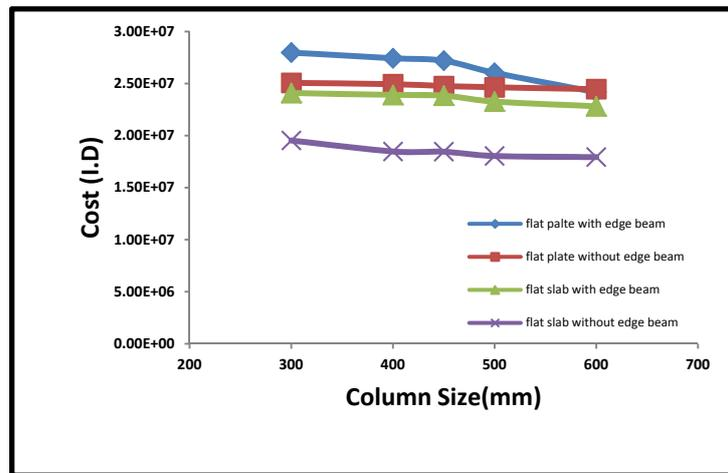
Figure (5) Effect of Column Size on the Slab Total Cost
