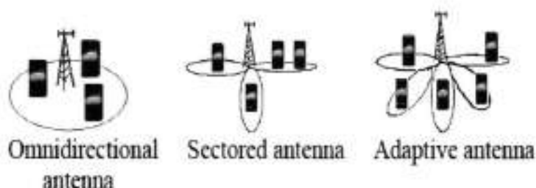
Fig. 1. Base Station Antenna Configurations
