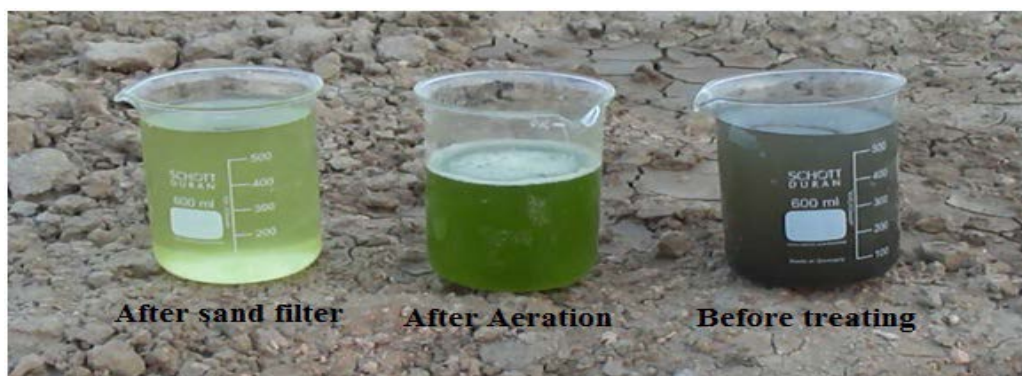
Figure (12) Picture show the difference in color without and with using sand filter.
