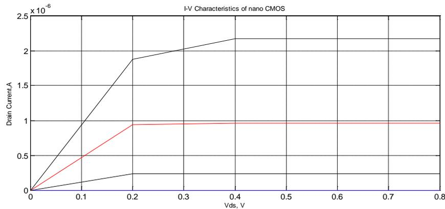
**Figure (10) Current voltage characteristics for different value of V<sub>gs</sub> in Nano (CMOS).**
