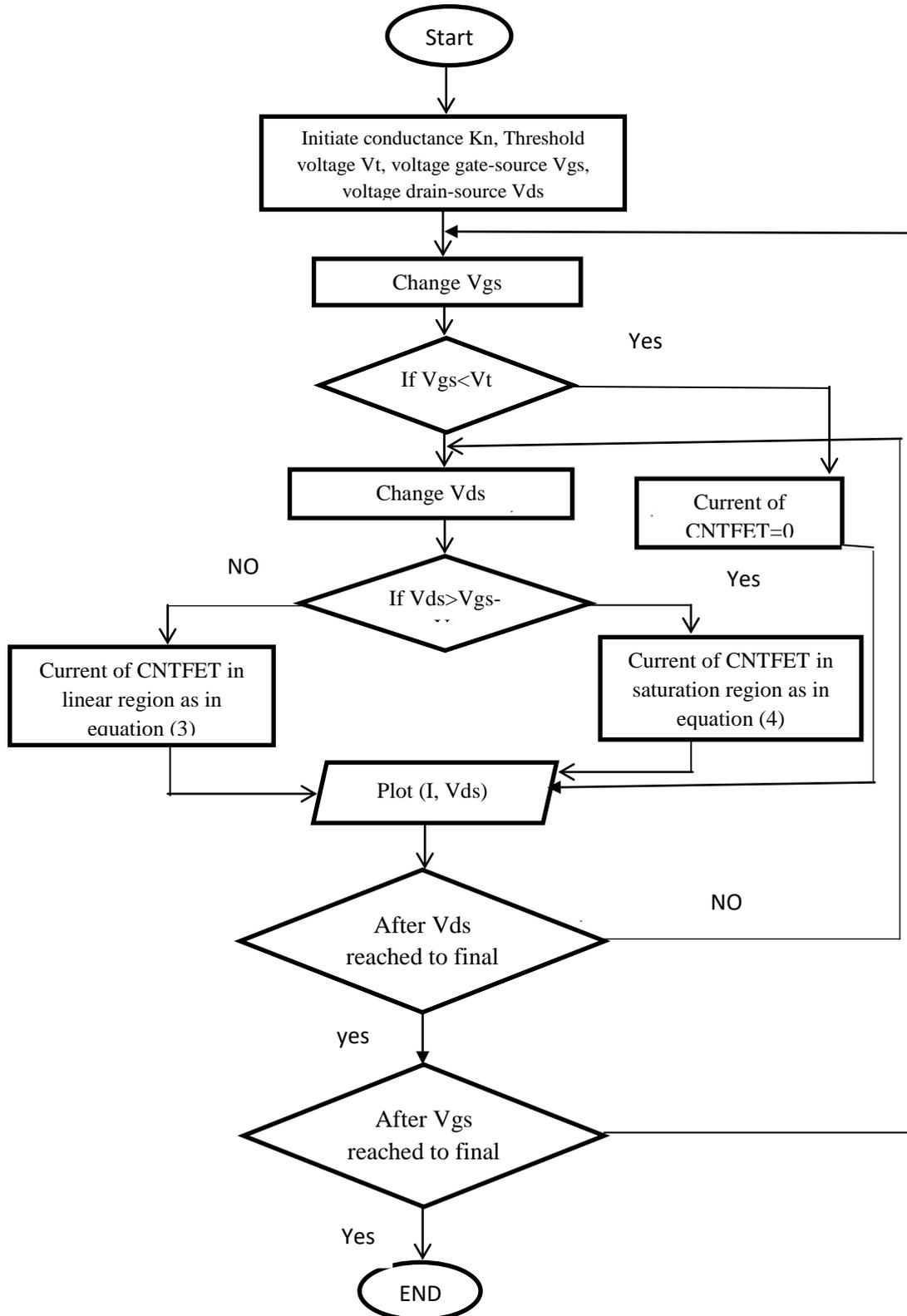
Figure (7) Flowchart of CNTFET Characteristics.
