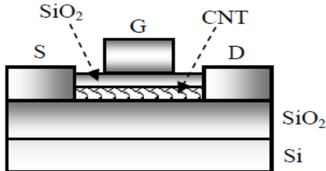
Figure (1) Schematic structures a CNTFET [10].
