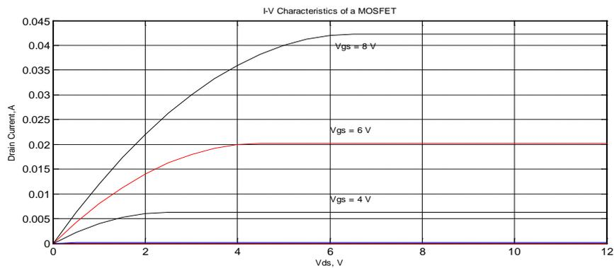
Figure (9) Current voltage characteristics for different value of  $V_{gs}$  in (MOSFET).
