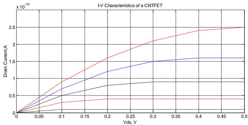
Figure (8) Current voltage characteristics for different value of  $V_{gs}$  in CNTFET.
