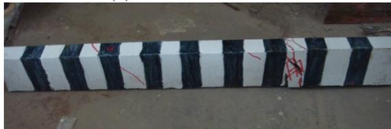
**Plate (9) Failure of Beam A1**
