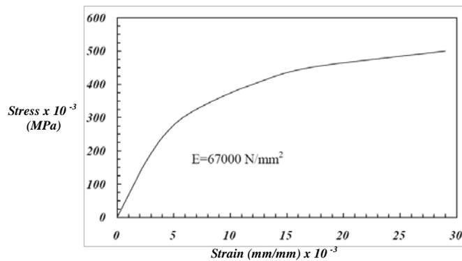
**Figure(1) Stress–Strain Curve of the Wire Mesh(12) 2-1-6 Mold.**
