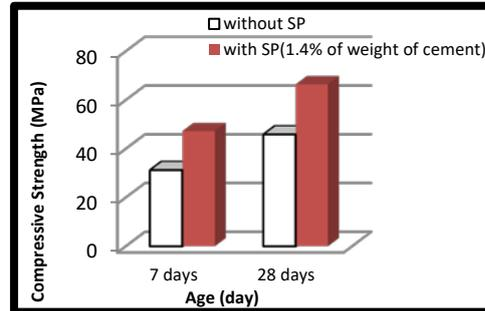
Figure (4) Improvement of Average Compressive Strengths of Mortar Mixes of Beams.
