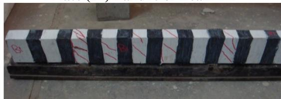
**Plate (12) Failure of Beam B1**
