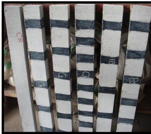
**Plate (2) Beams Strengthened with CFRP.**
