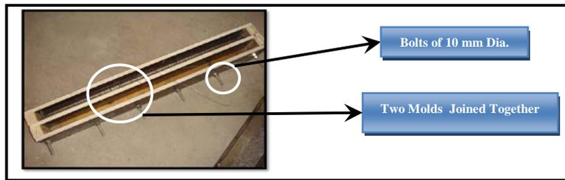
Plate (1) The Plywood Mold.
