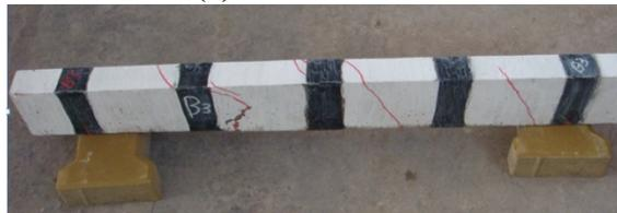
**Plate (10) Failure of Beam B3**
