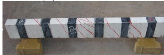
**Plate (11) Failure of Beam B2**
