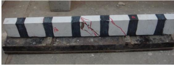
**Plate (8) Failure of Beam A2**
