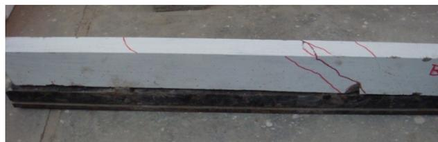
Plate (5) Failure of Beam BR (3units, without CFRP)
