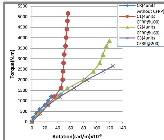
Figure(11) Torque-Rotation Relationships for Group C (Effect of Spacing of CFRP Strips).
