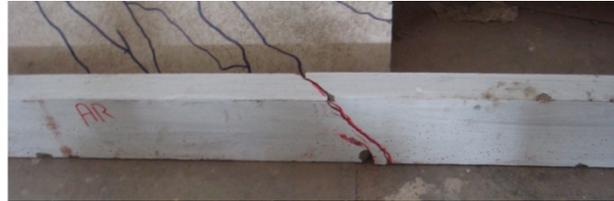
Plate (4) Failure of Beam AR (2units, without CFRP)
