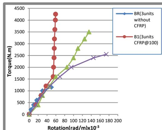
Figure (10) Torque-Rotation Relationships for Group B(Effect of Spacing of CFRP Strips).
