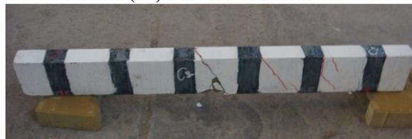
**Plate (14) Failure of Beam C2**
