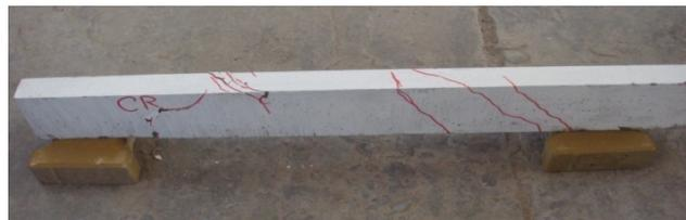
Plate (6) Failure of Beam CR (4units, without CFRP)
