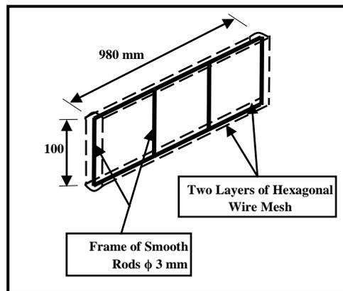
**Figure (2) Detail of Wire Mesh Unit.**
