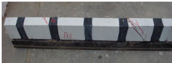
**Plate (7) Failure of Beam A3**
