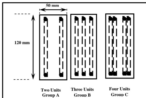
**Figure (3) Reinforcement of Cross Section of Beams.**
