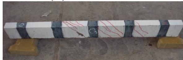
**Plate (13) Failure of Beam C3**
