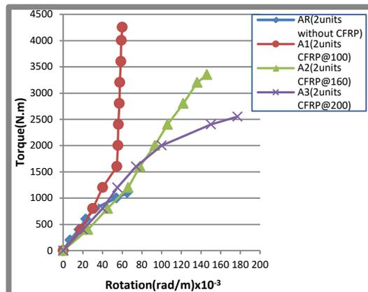
Figure(9) Torque-Rotation Relationships for Group A(Effect of Spacing of CFRP Strips).
