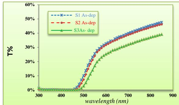
**Figure (1) Shows transmission spectrum of  $In_2S_3$  As-sprayed.**
