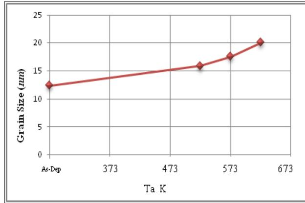
Figure (6). Variation in grain size of  $In_2S_3$  at different  $T_a$ .
