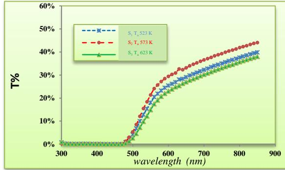
Figure (2) Shows transmission spectrum of  $In_2S_3$  at different  $T_a$ .
