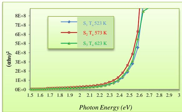
Figure (4)  $(\alpha h\nu)^2$  versus the photon energy ( $h\nu$ ) of  $In_2S_3$  layer with different ( $T_a$ ).
