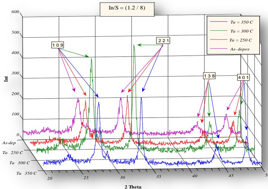
**Figure (5). XRD pattern for  $In_2S_3$  layer at different  $T_a$ .**
