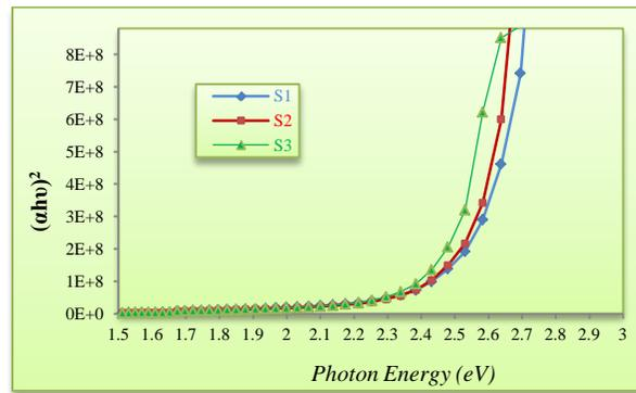
Figure (3)  $(\alpha h\nu)^2$  versus the photon energy ( $h\nu$ ) of  $In_2S_3$  layer as-sprayed at different thicknesses.
