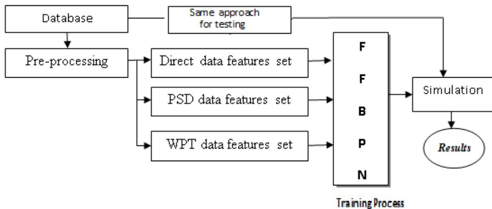
**Figure (1) The flow chart of the proposed procedure. After training the certain number of patterns by means of FFBPN, testing process is performed for recognition the feature vectors of the testing samples. The output of the training process is given to the testing stage, where the simulation process for testing features is performed. The output of the simulation process will determine the class.**
