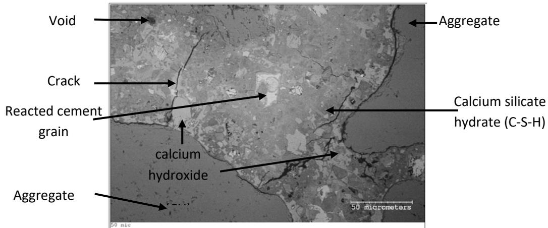
**Figure (1) SEM image of a Portland cement concrete (14 weeks old, w/c=0.4), with the view of microstructural component.**
