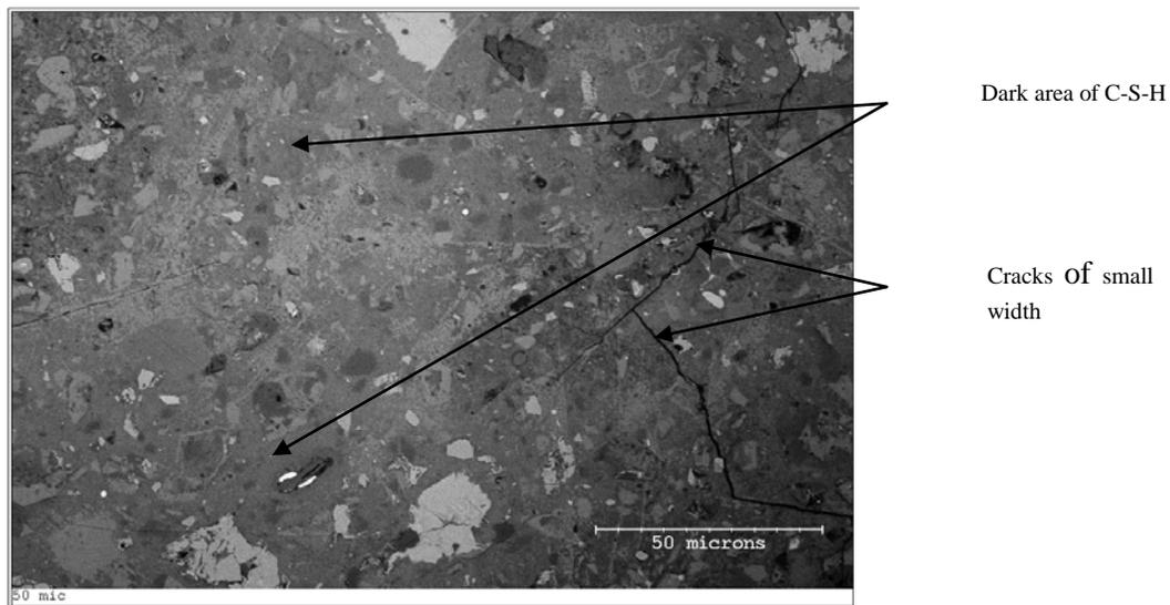
**b. SEM image of SF mortar showing dark and dense area of C-S-H, and absence of wide cracks.**
