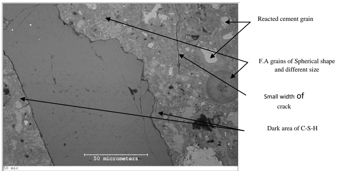
**a. SEM image of F.A mortar showing dense area of ITZ,
