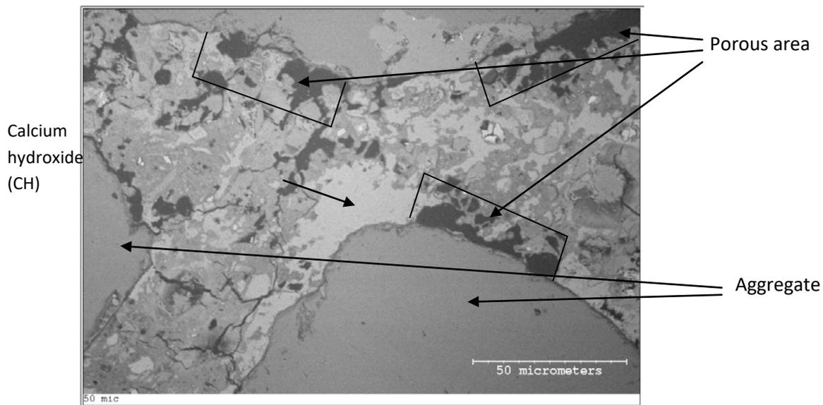
**Figure (2) SEM image of a Portland cement mortar (28-day old, w/c=0.5), with the view of ITZ.**
