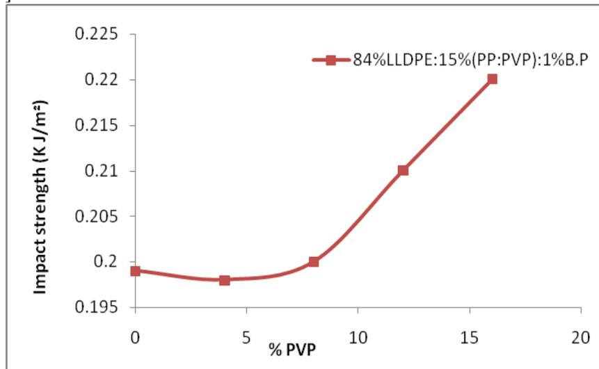
**Figure (10) Impact strength of [84%LLDPE:15%((100-X)%PP:%XPVP):1%B.P] as a function PVP content in the composites.**
