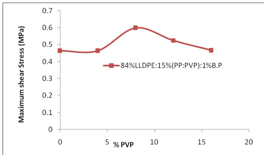
**Figure (8) Maximum shear stress of [84%LLDPE:15%((100- X)%PP:X%PVP):1%B.P] as a function of PVP in the composites.**
