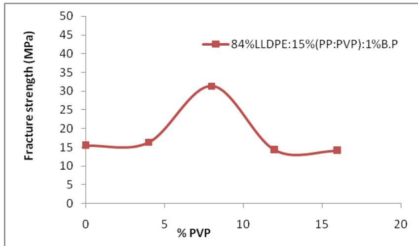
**Figure (3) Fracture strength of [84%LLDPE:15%((100- X)%PP:X%PVP:1%B.P] as a function of PVP content in the composites.**
