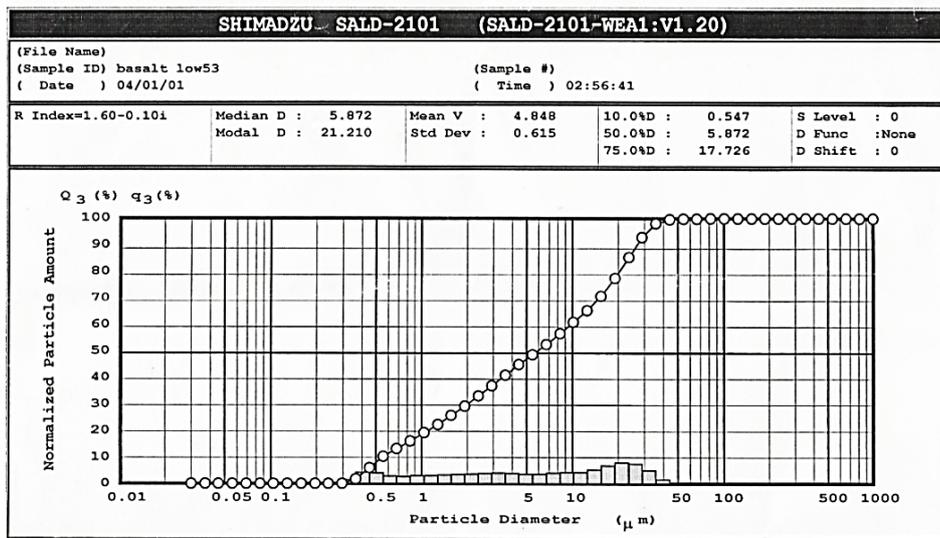
**Figure (1) shows particle size analysis of basalt.**
