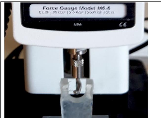
**Fig.(1): Shows pulling fiber during test**
