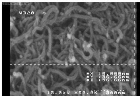
Figure (8) SEM image of PANI/1 wt% CNT Composite magnified 60000 times.
