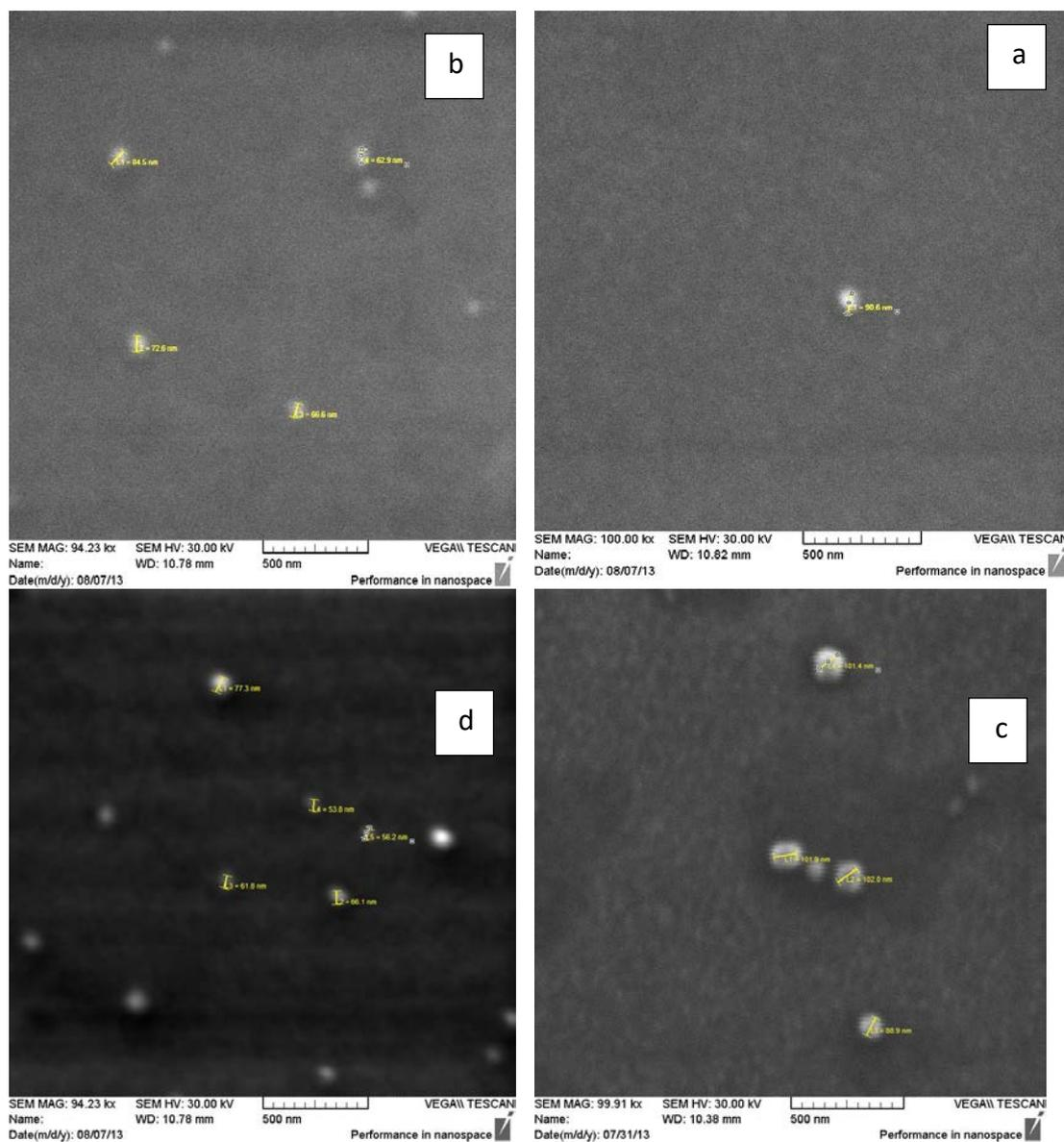
**Figure (3) SEM image of Ag NPs prepared at 1.06  $\mu\text{m}$  laser wavelength and different laser energy (a-100, b-200 and c-600 d-800) m J and 100 pulse.**
