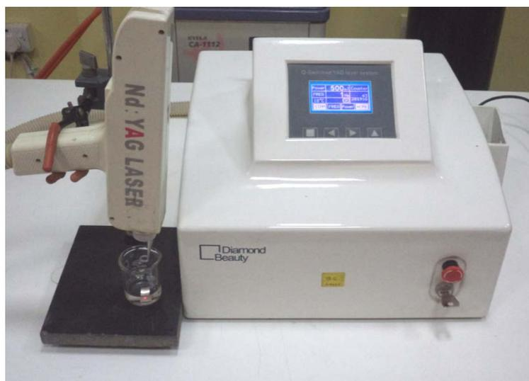
**Figure (1) Experimental setup for nanoparticles synthesis by PLAL.**
