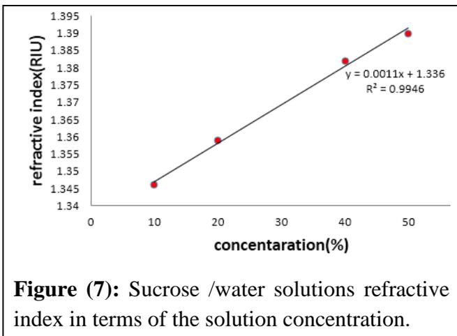
**Figure (7):** Sucrose /water solutions refractive index in terms of the solution concentration.
