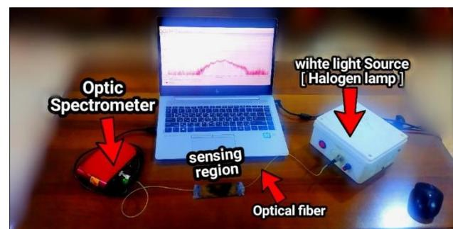
**Figure (2): The experimental setup of SPR multi-mode fiber sensor.**
