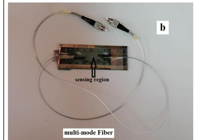
**Figure (5):** (a) Single-mode no core fiber sensor (b) Multi-mode no core fiber sensor.
