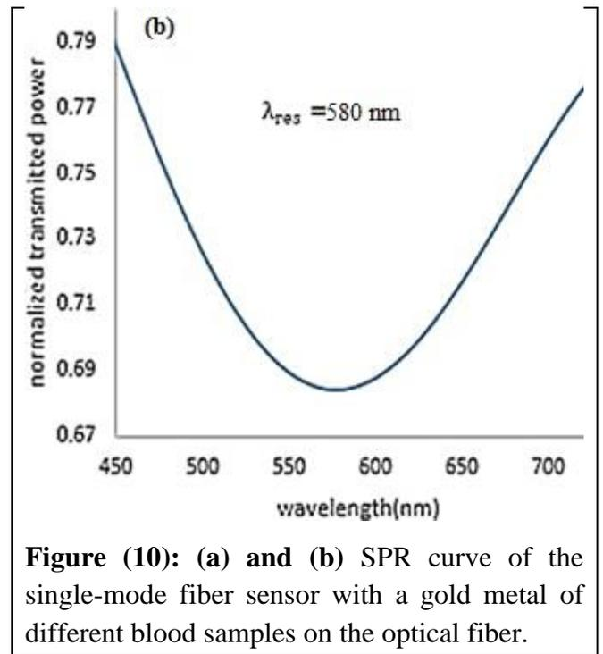
**Figure (10): (a) and (b) SPR curve of the single-mode fiber sensor with a gold metal of different blood samples on the optical fiber.**
