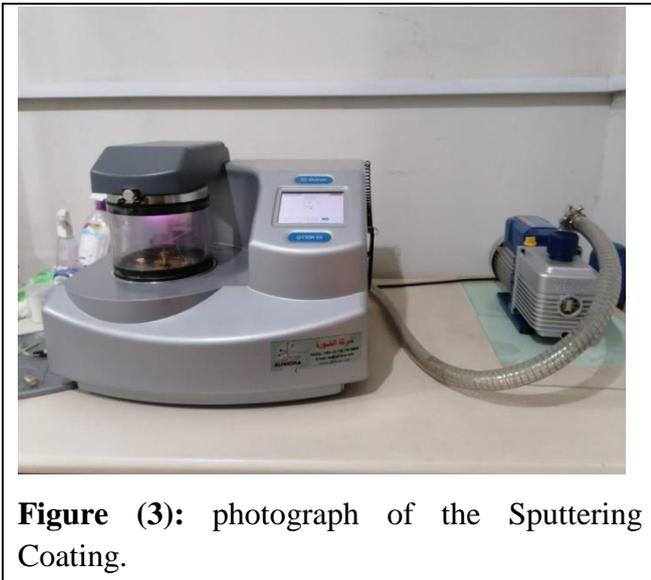
**Figure (3):** photograph of the Sputtering Coating.
