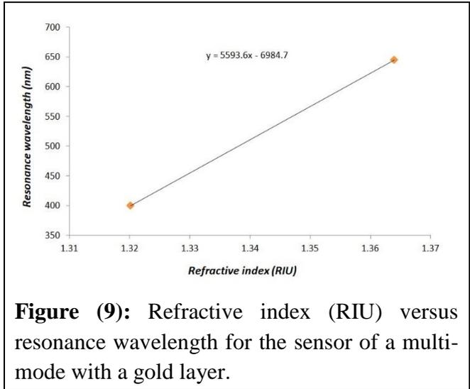
**Figure (9):** Refractive index (RIU) versus resonance wavelength for the sensor of a multi-mode with a gold layer.
