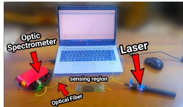
**Figure (1): The experimental setup of SPR single mode fiber sensor.**
