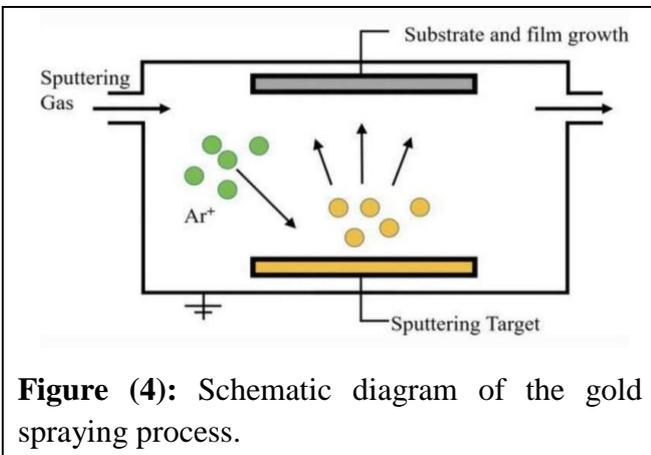
**Figure (4):** Schematic diagram of the gold spraying process.
