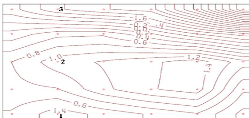
Figure (5): pressure distribution over trough surface obtained from experimental work (bar) [6].
