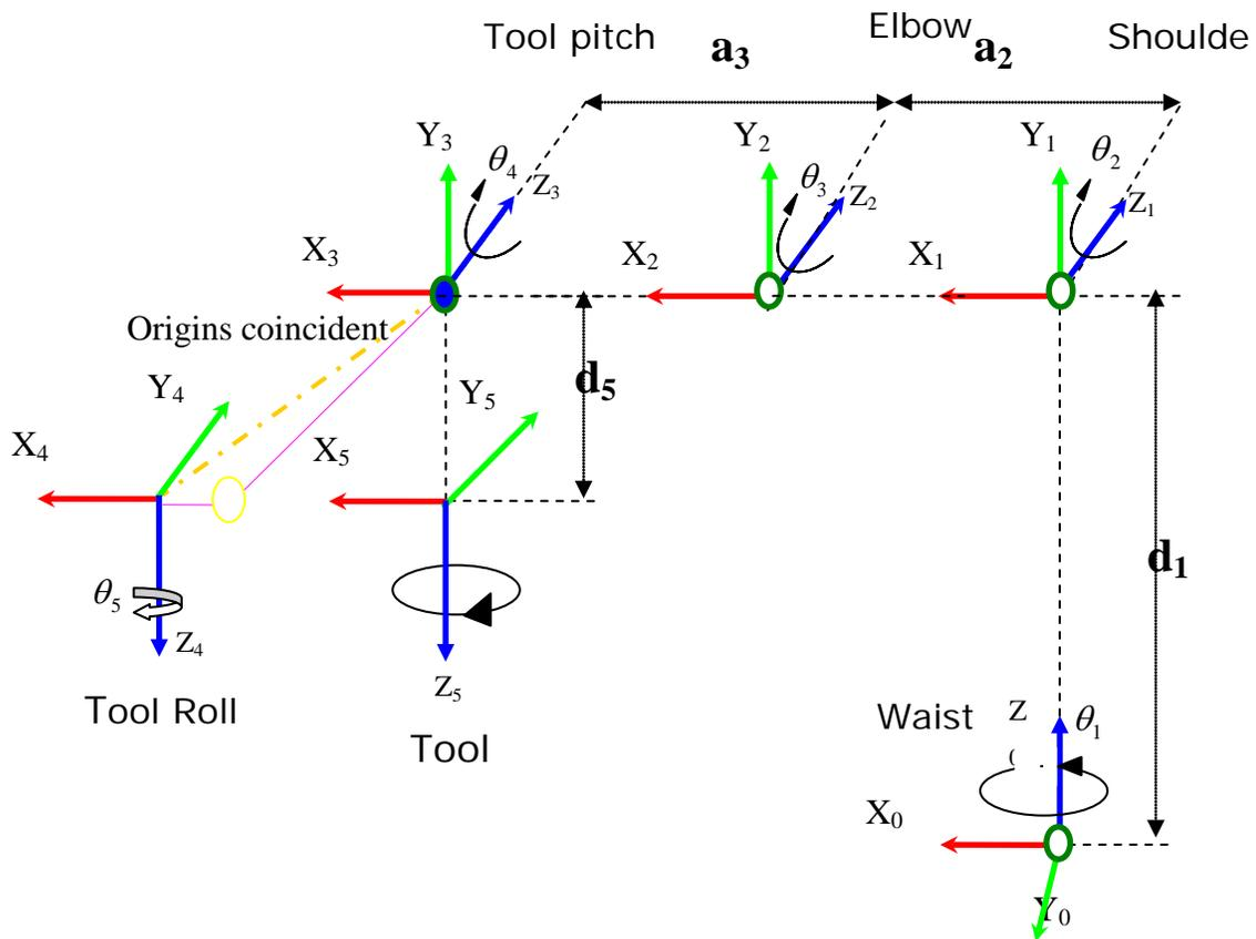
Figure (1) link coordinates of a 5DOF Robot manipulator [13].
