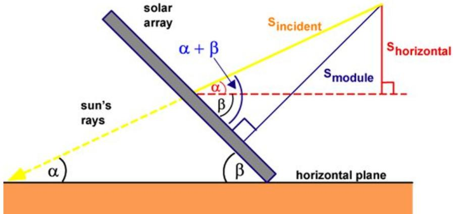
Figure (1) Tilting the module to the incoming light reduces the module output.
