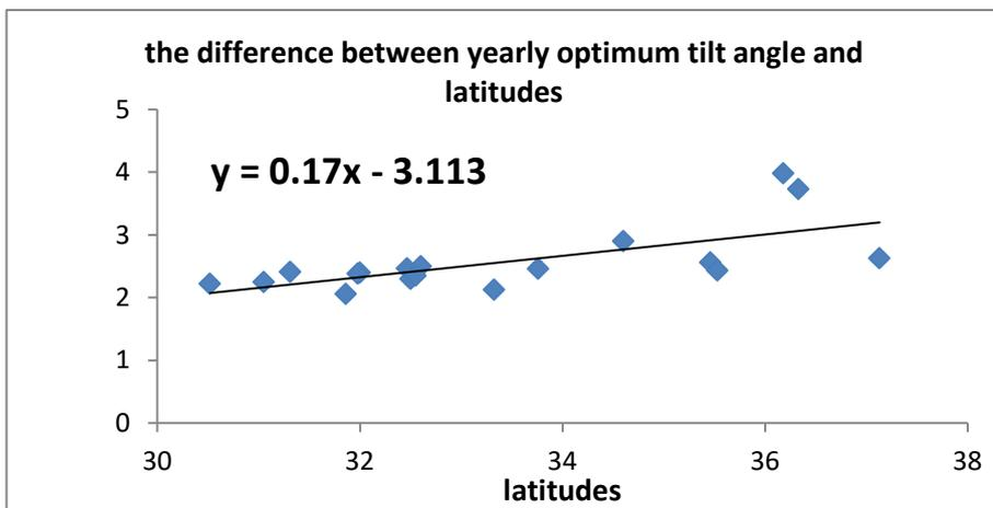
Figure (5) Linear relationship between yearly optimum tilt angle and latitudes.
