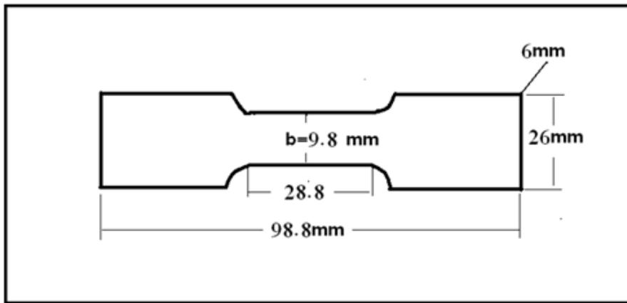
**Figure (1) Dimensions of tensile specimen.**
