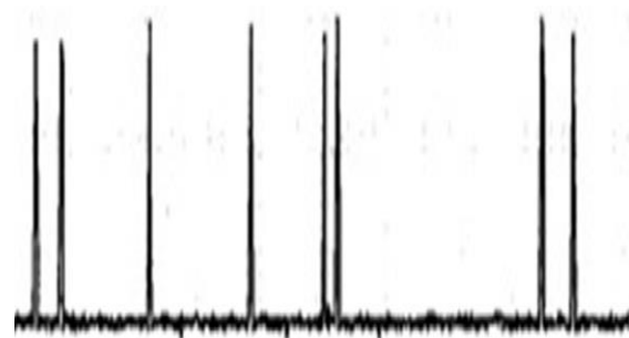
Fig.(3): The random time of arrival of consecutive photons of attenuated laser source [7]
