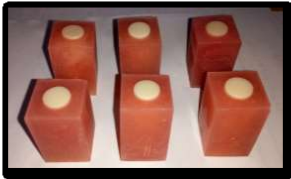
Figure (2) Zirconia discs were embedded in an acrylic mold
