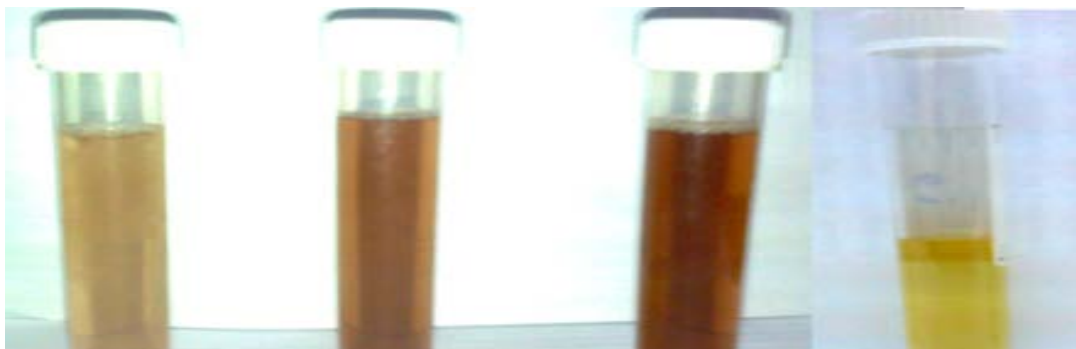
Figure (2) photo shows formation stages Ag nanoparticles prepared by \text{AgNO}_3 with CTAB with oxalic acid.
