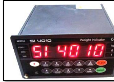
Figure (10) Digital weighing indicator.
