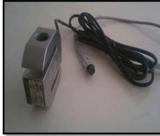
Figure (9) Load cell.
