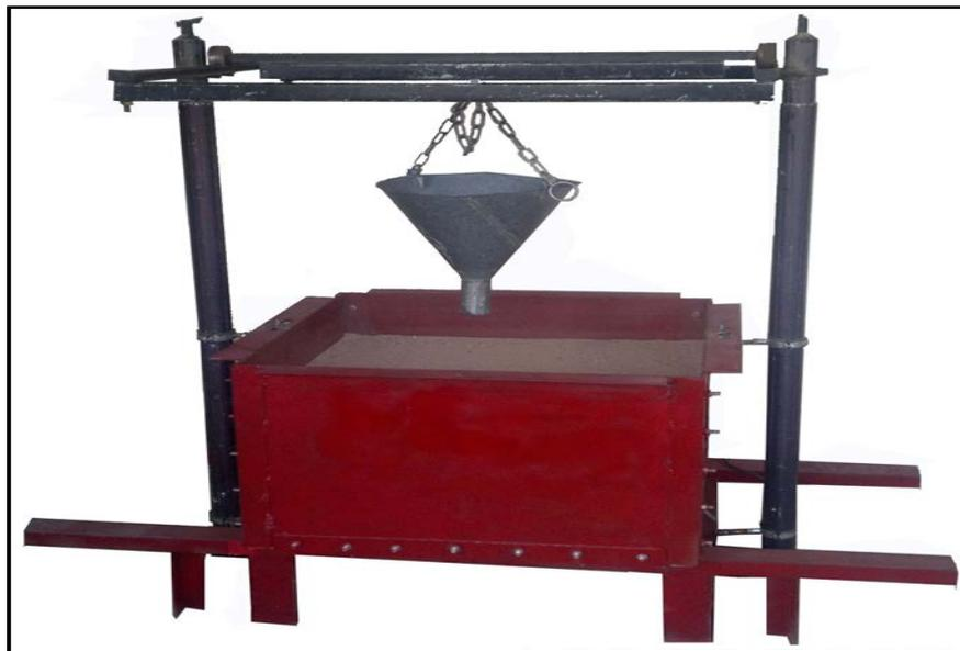
**Figure (7) Raining frame used for controlling density.**
