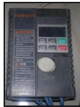
Figure (12) AC drive (Regulator of speed).
