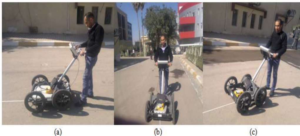
Figure (2) Fieldwork inspection with GPR antenna frequencies using: (a) 250 MHz, (b) 500 MHz, and (c) 800 MHz
