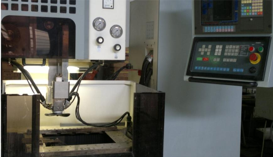
**Figure (2) WEDM Cutting Machine**
