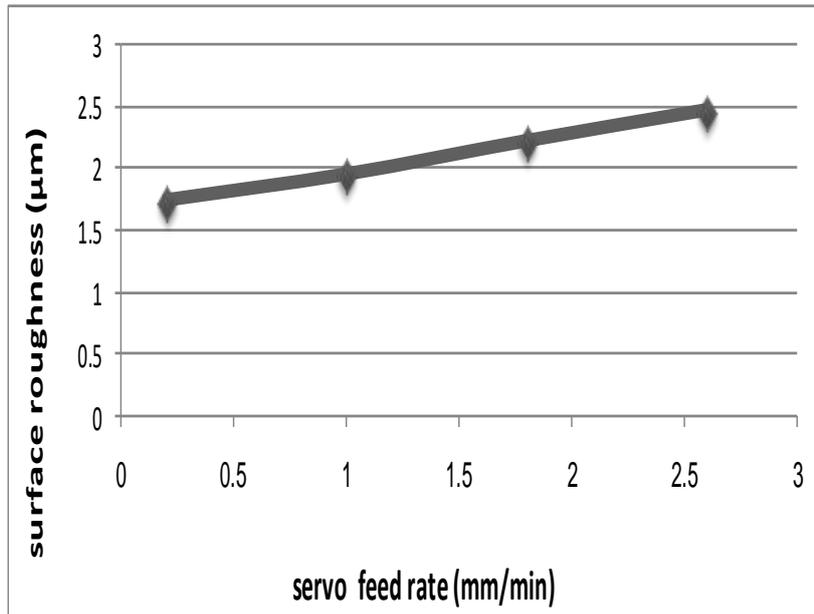
Figure (8) Effect of servo feed rate on surface roughness using brass wire.
