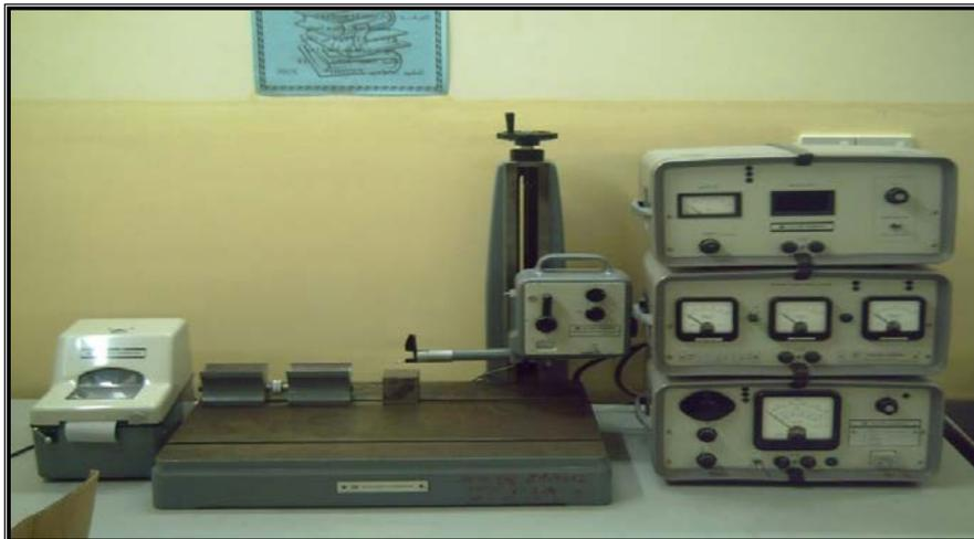
**Figure (3) Talysurf4 (roughness measurements instrument)**
